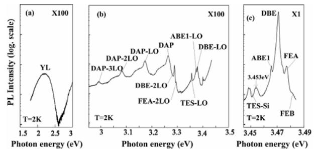
Fig. 9: LT-PL measurements of the yellow (left), DAP (center) and exciton (right) spectral ranges. Attention: different scales!
