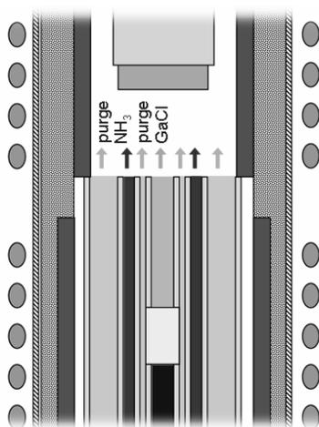
Fig. 4: Concentric reactor inlet geometry.
