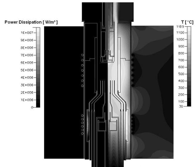
Fig. 2: Numerical simulation of the temperature distribution in the reactor. Power dissipation (left) and temperature distribution (right) are shown (not drawn to scale).
