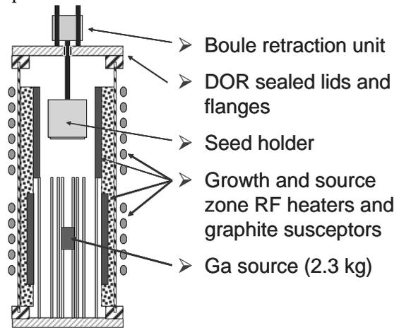
Fig. 1: Schematic sketch of the VHVPE growth reactor detailing its components (not drawn to scale).
