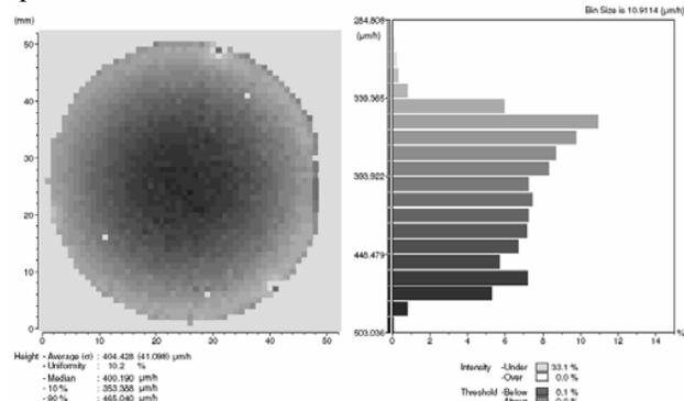
Fig. 6: WLI growth rate map over a 2 inch layer. 400  $\mu\text{m}/\text{h}$  with a uniformity of 10.2% were achieved.
