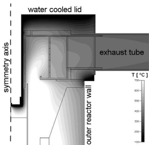
Fig. 5: Numerical simulation of the exhaust collector temperature distribution under process conditions (cross section not drawn to scale).
