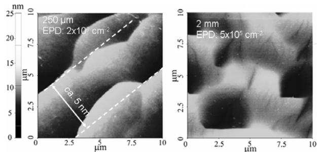
Fig. 8: AFM scans of 10x10  $\mu\text{m}$  areas of a 250  $\mu\text{m}$  (left) and a 2 mm (right) thick layer. Height scale identical in both pictures.
