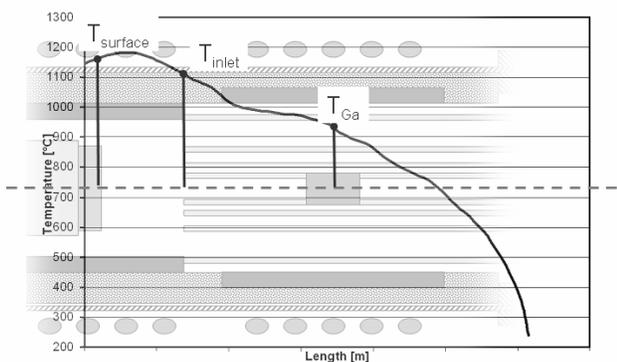
Fig. 3. Temperature scan along the reactor axis (from numerical simulation).
