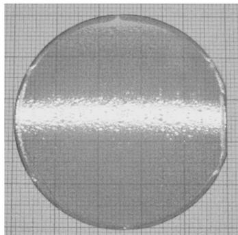
Fig. 7: Photograph of a 130  $\mu\text{m}$  thick layer grown at 250  $\mu\text{m}/\text{h}$ .
