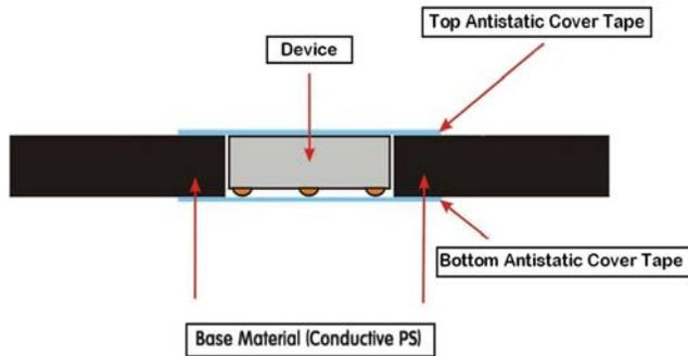
**Figure 7. Illustration of a solder bumped die packaged in MicroTape tape and reel format.**
