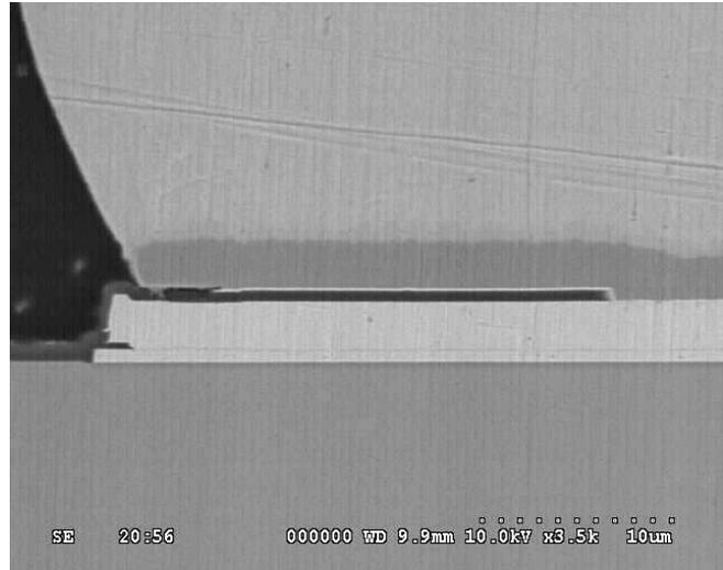
**Figure 2. Image of solder and barrier layer, which prevents diffusion of the Au and Sn**
