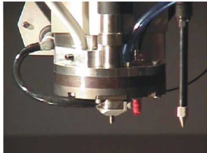
**Figure 3. Laser dispense system for individual solder ball placement.**
