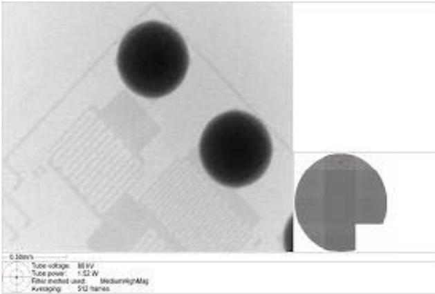
**Figure 4. X-Ray analysis of individually placed solder balls.**
