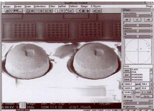
**Figure 5. Product testing on solder bump utilizing a cascade pyramid probe.**
