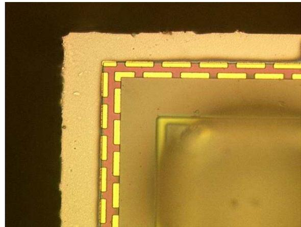
**Figure 6. Laser dice of a solder bumped part demonstrated minimal kerf width and significantly reduced dice times. Courtesy of ALSI.**
