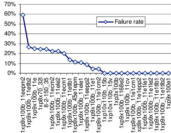
Figure 3: Failure rate after mechanical stress for various power cell designs.
