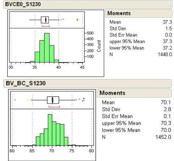
Figure 2: Distribution of BVce0 and BVbc0 for 1450 measurements across 80 wafers.
