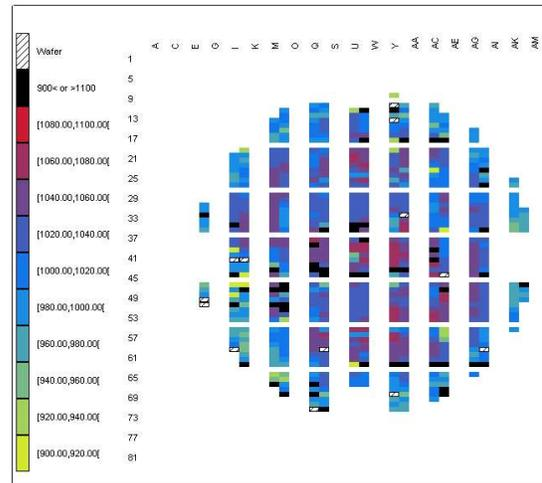
Figure 6: on-wafer mapping of the collector current at fixed base current (25mA) for 35W power bars. (716 devices tested). Mean = 950mA - std. Dev. = 33mA
