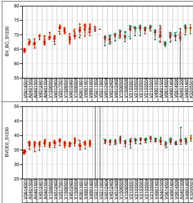
Figure 1: Trend-chart of base-collector (top) and emitter-collector (bottom) breakdown voltage (PCM - 2x30micron device).
