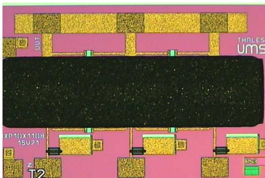
Figure 5: Picture of a 15-W power bar.
