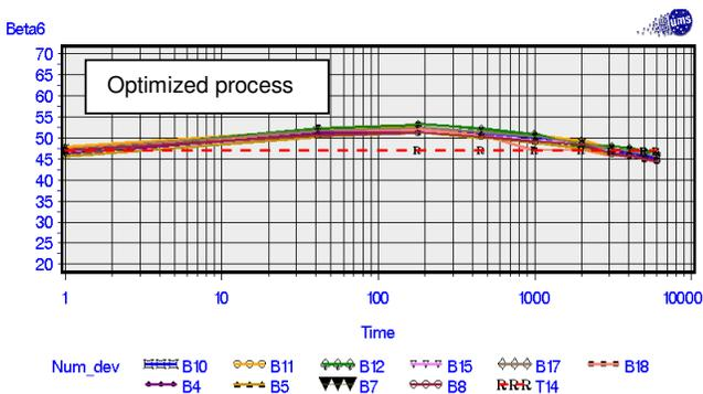
Figure 9: Current gain versus time (hours) of power cells under accelerated aging conditions ( $T_j = 223^\circ\text{C}$ ). Optimized process. (Red dashed lines are un-stressed reference devices).
