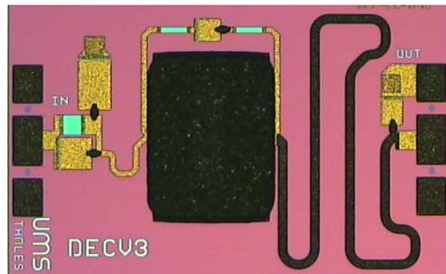
Figure 7: Photograph of a pre-matched power cell for reliability testing.
