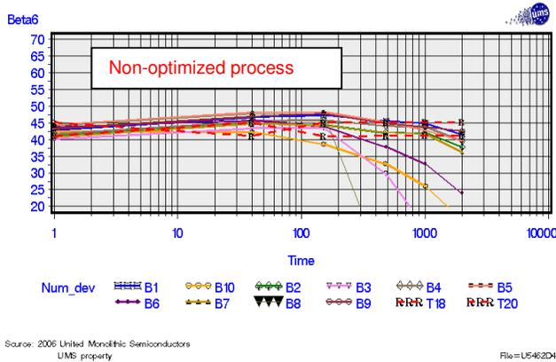
Figure 8: Current gain versus time (hours) of power cells under accelerated aging conditions ( $T_j = 223^\circ\text{C}$ ). Non-optimized process. (Red dashed lines are un-stressed reference devices).
