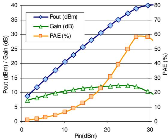
Figure 4: Power performance of a 1,800- $\mu\text{m}$  emitter periphery transistor -  $f=3.1\text{GHz}$  -  $V_{ce}=20\text{V}$  - B class.
