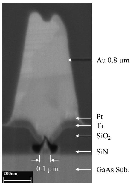
Fig. 4. SEM cross-section of FET gate region.
