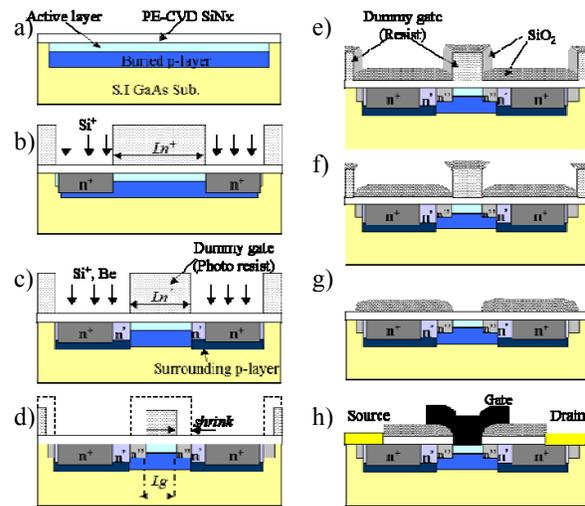
Fig. 1. Main fabrication sequence of SRD Process.
