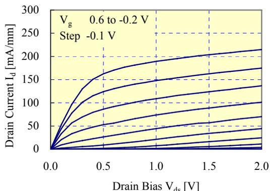
Fig. 6. I-V Characteristics of MESFET.
