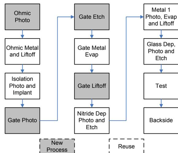
**Figure 1.** pHEMT process flow highlighting new versus reused process modules.
