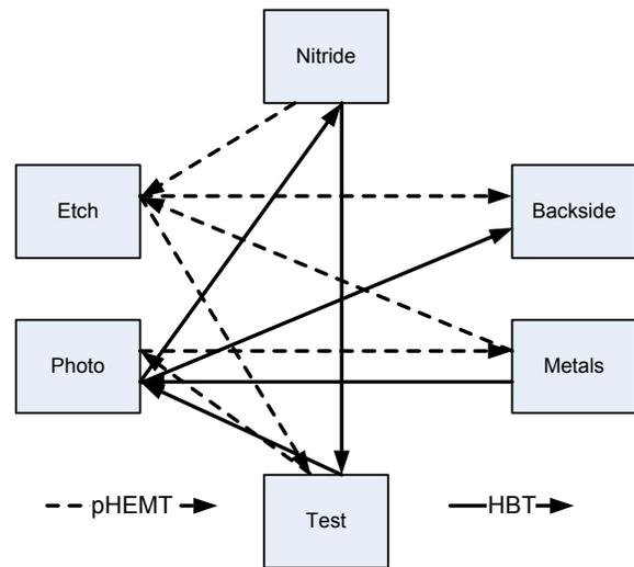
**Figure 2.** Illustration showing two different technologies (pHEMT and HBT) utilizing the same wafer fab “job shop.”
