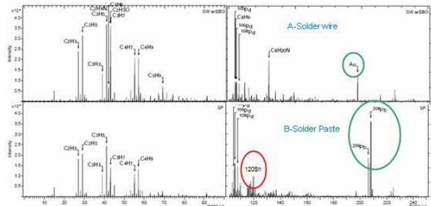
Fig.5 is the XPS spectrum of the die flag with SP and WB. Oxygen, carbon, tin, lead, palladium, gold and small amounts of sulfur and silicon were apparent. From analysis
