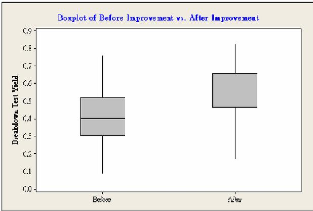
Figure 8. Breakdown yield comparison before and after the process and epitaxial material improvement
