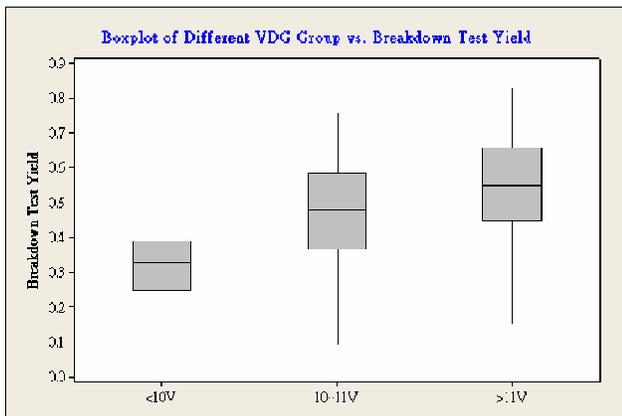
Figure 5. Higher PCM4 Breakdown voltage (VDG) corresponds to lower breakdown screening yield. The PCM4 breakdown voltage was defined as  $I_{ds}$  at 1mA/mm measured on a device of 1gate finger with 75um gate width.
