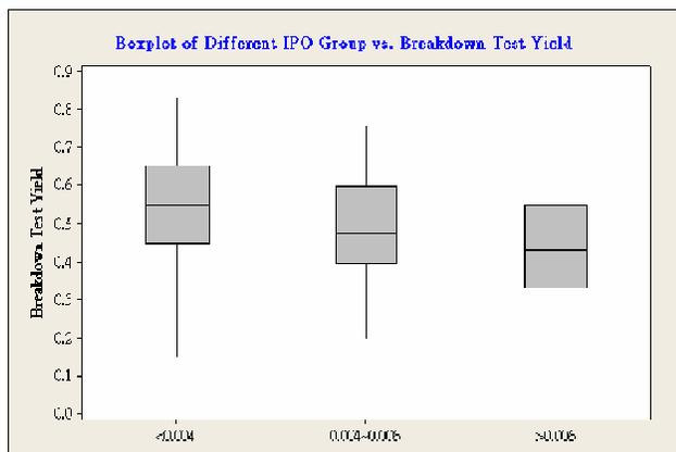
Figure 6. Lower PCM 3-terminal leakage current (IPO) corresponds to lower breakdown screening yield. The PCM 3-terminal leakage current was measured on a device of 1gate finger with 75um gate width at  $V_{gs}=-2V$  and  $V_{ds}=1.5V$ .
