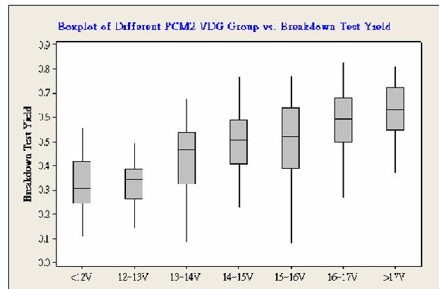
Figure 7. The correlation of the PCM2 VDG values and the breakdown screening yield distribution.
