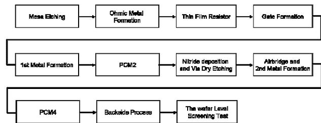
Figure 1. Process Flowchart of WIN 0.15um power pHEMT
