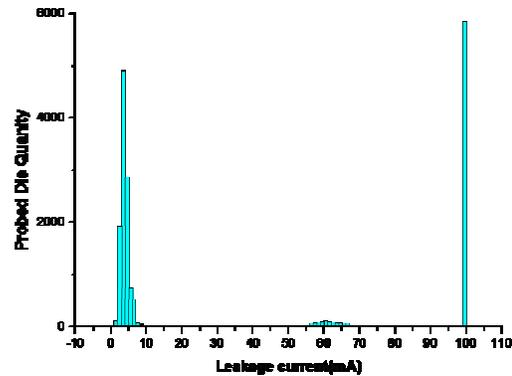
Figure 4. The histogram of leakage current at the breakdown-screening test
