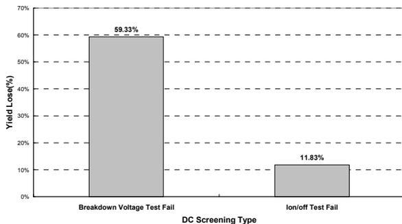
Figure 2. The yield loss of the two DC screening parameters
