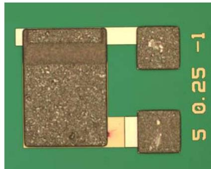
Figure 5. Photograph of one of the capacitors tested. Note the splatter on the lower contact pad as evidence of failure. The layer spacings are coded on the right side CB-OV=5  $\mu\text{m}$ , OV-Post=0.25  $\mu\text{m}$ , and Post-Bridge=1  $\mu\text{m}$ . The top plate is fully plated and the airbridge connects to the pad in the top of the photo.
