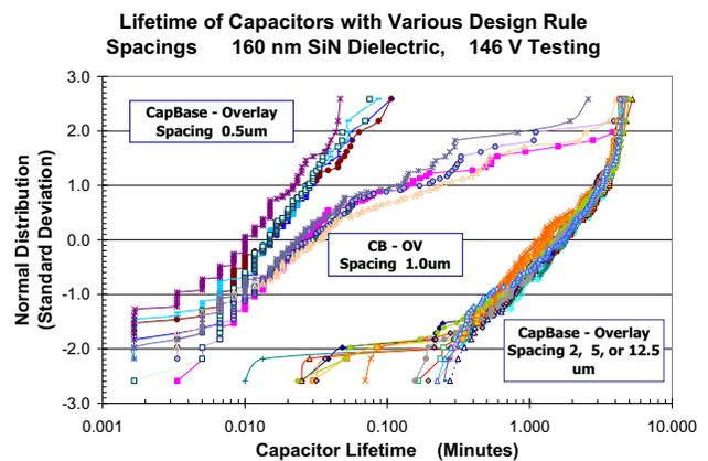
Figure 2. Lifetime results from capacitors fabricated utilizing 160 nm dielectric thickness. Discrete steps in the distribution for short lifetimes result from the 0.1 sec resolution chosen for the test program.
