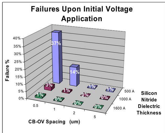
Figure 7 Early Failures. Capacitors that were initially functional but failed in the first 0.2 sec of voltage application.
