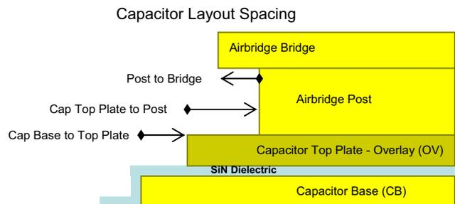
Figure 1. Capacitor layout design rule spacing dimension identification.
