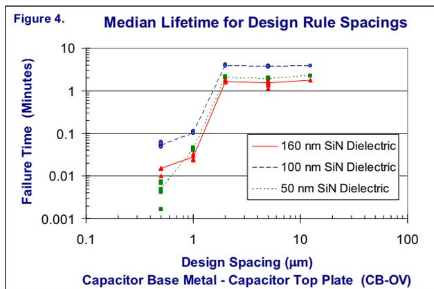
Figure 4. Capacitor median lifetime for the range of design rule spacings. Each of the nitride thickness shows a similar trend with reduced lifetime below 2  $\mu\text{m}$ . The difference in lifetime for the different nitride thickness result from slight differences in applied electric field, in thickness from the nominal, and in the roughness of the base metal which acts as a linear subtraction from the nitride thickness.
