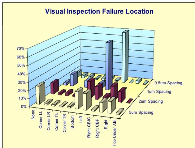
Figure 6. Failure locations of the 4000 capacitors from a wafer with 160 nm SiN dielectric.
