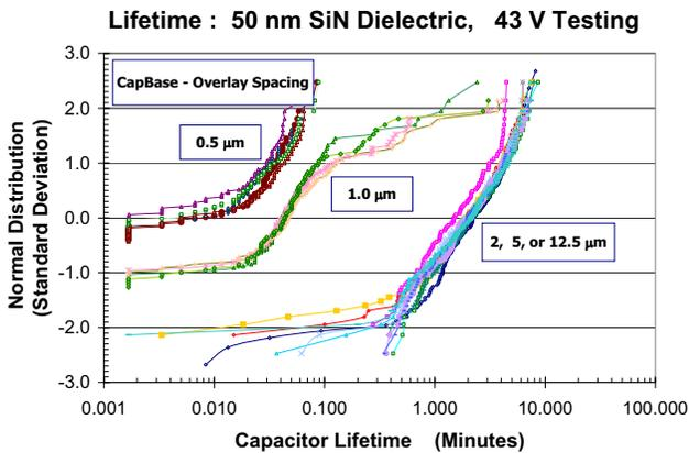
Figure 3. Lifetime results from capacitors fabricated utilizing 50 nm dielectric thickness.
