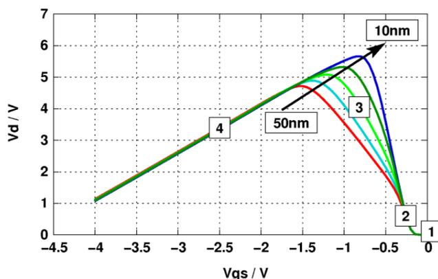
**Figure 6: Device Simulation: influence of the distance between channel and super lattice and breakdown voltage**
