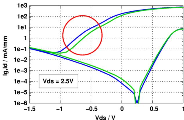
**Figure 2: Device simulation: drain and gate leakage currents for 100nm gate length HEMTs with different distances between Schottky contact and channel**
