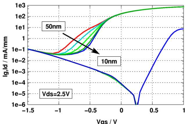
**Figure 5: Device simulation: gate and drain leakage current with different distances between channel and super lattice**
