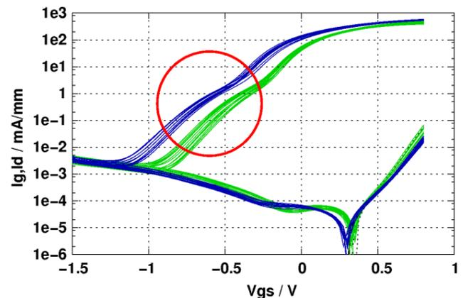
**Figure1: Measurement: drain and gate leakage current for 100nm gate length transistors with two different distances between Schottky contact and channel**
