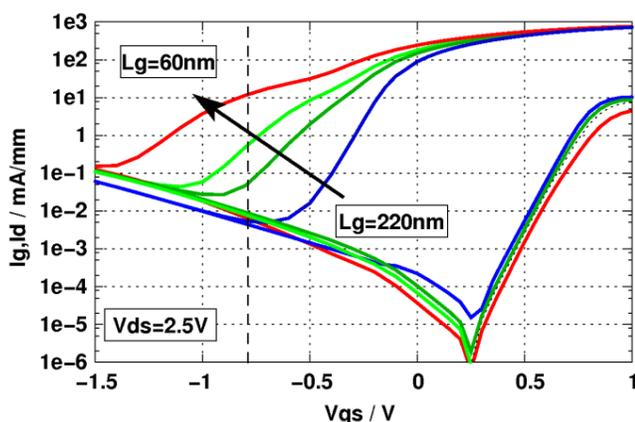
**Figure 3: Device simulation: drain and gate leakage current for different gate lengths**
