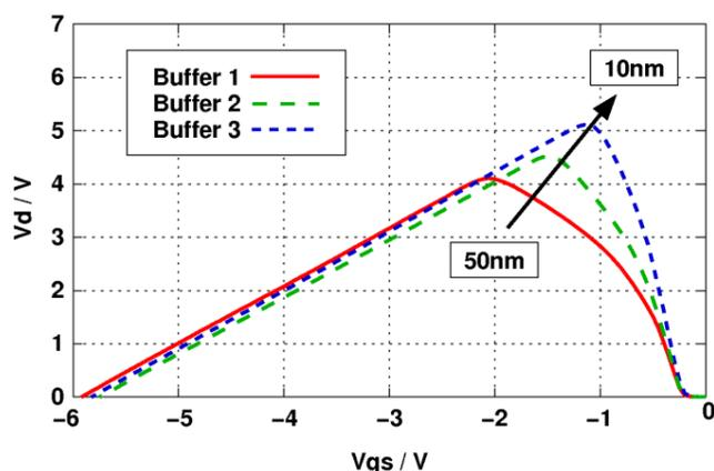
**Figure 7: Measurement: breakdown voltage for three different distances between channel and super lattice and a gate length of 100nm**
