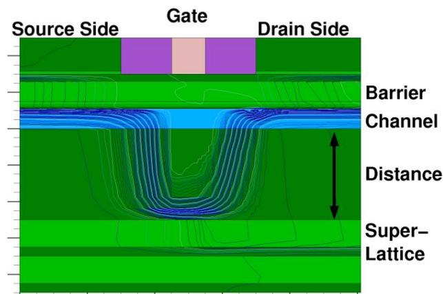
**Figure 4: Device simulation: current flow lines for  $L_g=100nm$ ,  $V_{ds}=2.5V$  and  $V_{gs}=-0.8V$**
