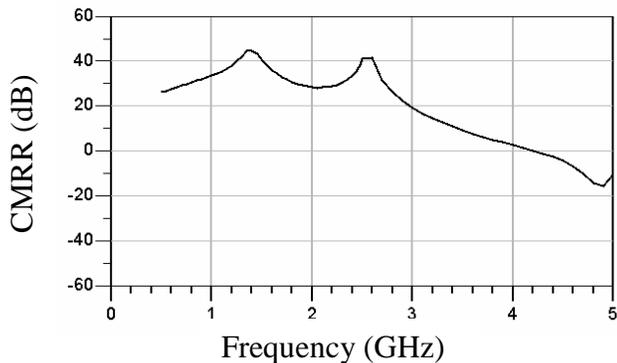
Figure 5. Common mode rejection ratio (dB) of ISM balun of nominal design over frequency 500 MHz and 5GHz.
