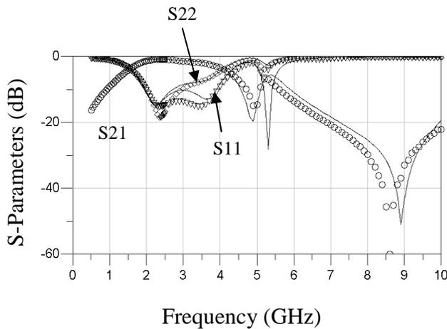
Figure 3. Comparison of measured (circle, triangle and square) and simulated (lines) insertion loss S21, and input, S22, and output, S11 return losses respectively, of ISM balun.
