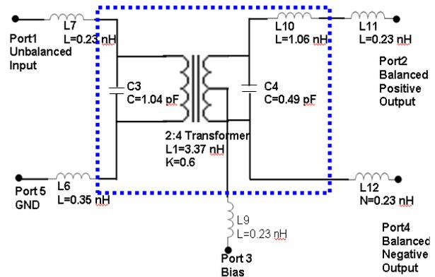
Figure 1. Schematic of 4:1 balun with wirebond inductors and matching elements.
