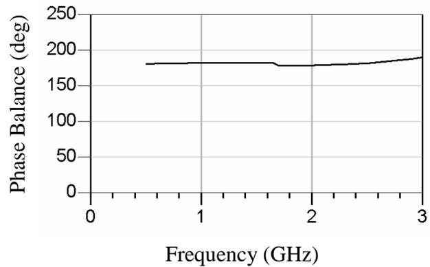
Figure 4 . Phase balance of balun over frequency range 500 MHz to 3 GHz..
