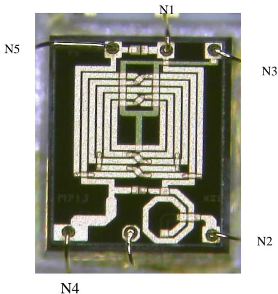
Figure 2. 4:1 ISM Balun die mounted for testing.
