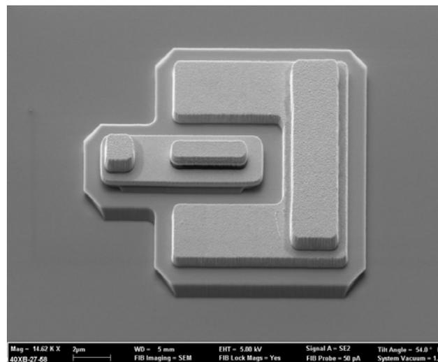
Figure 1: SEM-picture of an InP-DHBT before planarization.
