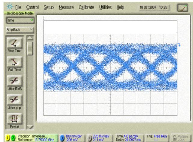
Figure 6: 110 Gbit/s single-ended data signal used for driving the DEMUX-IC.
