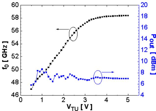
Figure 6: Oscillation frequency  $f_0$  and single-ended output power  $P_{out}$  vs. tuning voltage  $V_{TU}$ .
