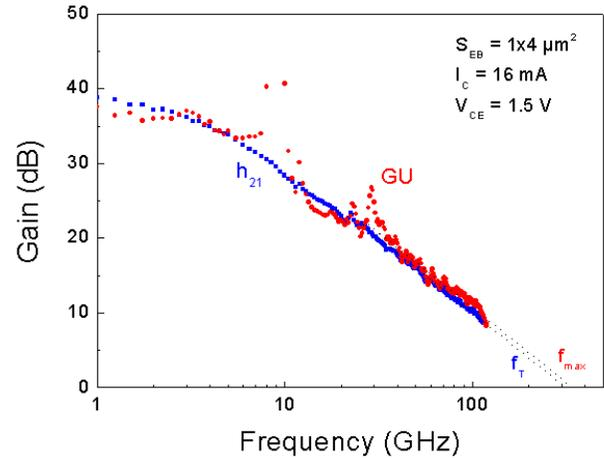
Figure 4: RF-properties of a  $1 \times 4 \mu\text{m}^2$  InGaAs/InP DHBT.
