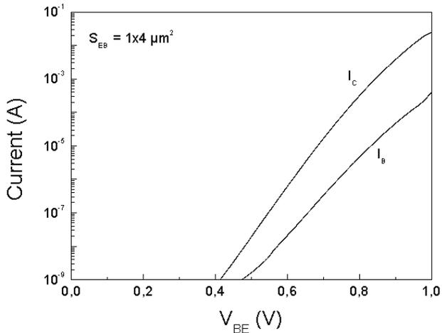
Figure 2: Typical Gummel-plots of InGaAs/InP DHBTs
