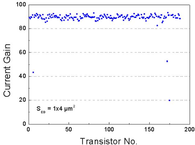
Figure 3: Current gain variation across a 3" wafer.
