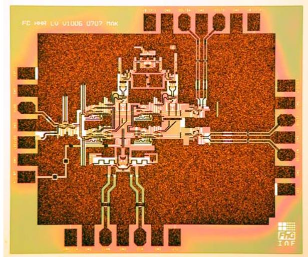
Figure 5: Chip photograph of the realized DEMUX circuit. The chip size is  $1.75 \times 1.5 \text{ mm}^2$ .
