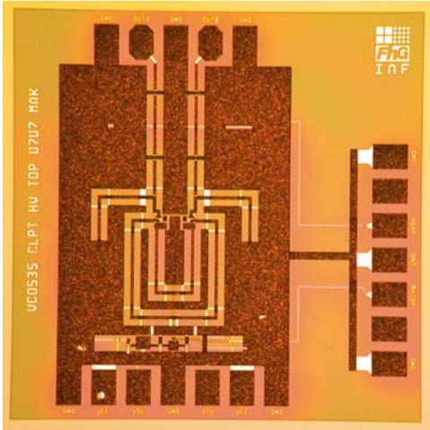
Figure 5: Chip photograph of an InGaAs/InP DHBT-based VCO. The chip-size is:  $1.25 \times 1.25 \text{ mm}^2$ .
