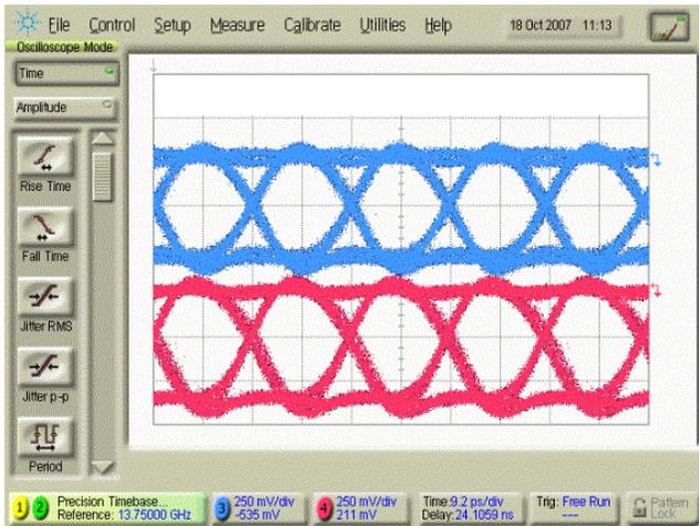
Figure 7: 55 Gbit/s demultiplexed data for a 110 Gbit/s input signal.
