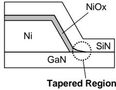
**Fig. 9** Schematic cross-sectional view of tapered gate shape in AlGaIn/GaN HEMTs.
