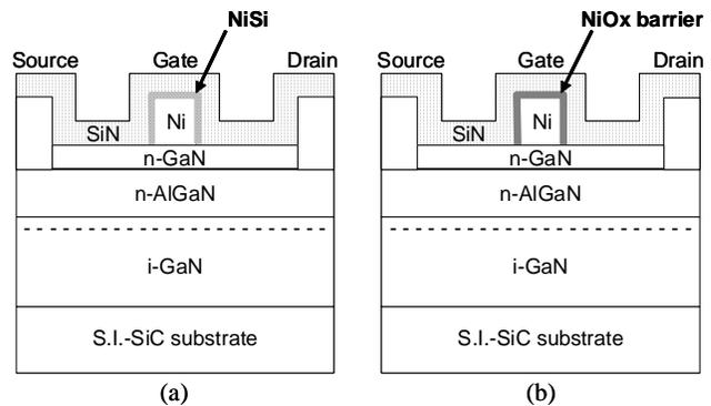
Fig. 1 Schematic cross-sectional view of (a) conventional and (b) our proposed AlGaN/GaN HEMTs.
