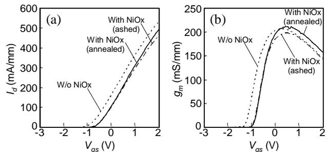
Fig. 8 (a)  $I_d-V_{gs}$  and (b)  $g_m-V_{gs}$  characteristics of annealed, ashed and conventional AlGaIn/GaN HEMTs.
