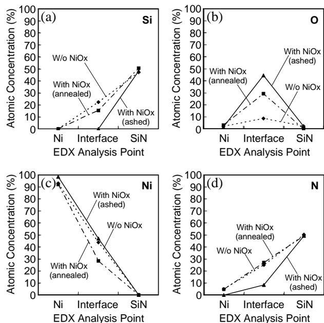
Fig. 4 Atomic concentration measured by EDX. Results are compiled for each element: (a)Si, (b)O, (c)Ni and (d)N.
