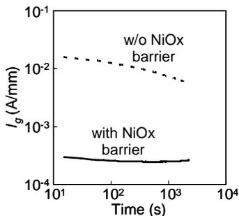
**Fig. 11** On-wafer DC stress test at 150°C.  $V_{ds}$  and  $V_{gs}$  were 50 V and -5V, respectively.  $I_g$  was monitored during this test.
