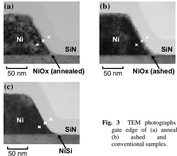
Fig. 3 TEM photographs of gate edge of (a) annealed, (b) ashed and (c) conventional samples.
