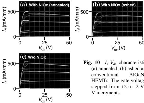
**Fig. 10**  $I_d$ - $V_{ds}$  characteristics of (a) annealed, (b) ashed and (c) conventional AlGaIn/GaN HEMTs. The gate voltage was stepped from +2 to -2 V in -1 V increments.
