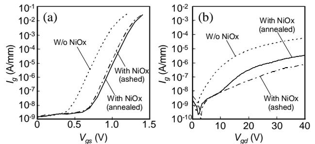
Fig. 7 (a) Forward and (b) reverse gate leakage characteristics of annealed, ashed and conventional AlGaIn/GaN HEMTs.
