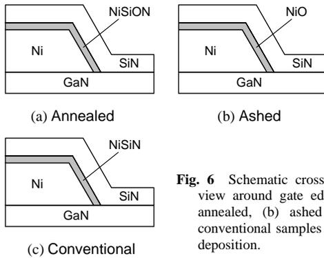
Fig. 6 Schematic cross-sectional view around gate edge of (a) annealed, (b) ashed and (c) conventional samples after SiN deposition.
