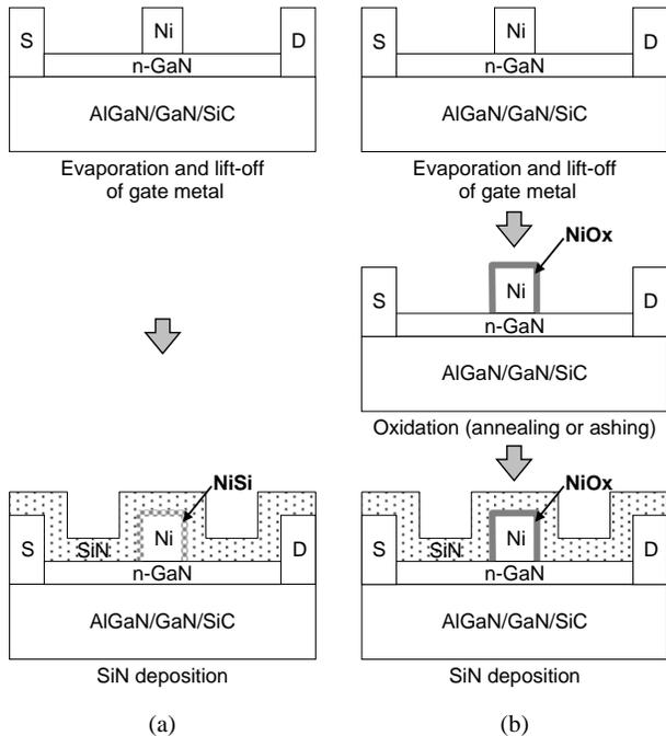
Fig. 2 Process flow diagrams of (a) conventional sample and (b) Ni-gate-oxidized sample.
