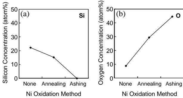
Fig. 5 (a) Silicidation ratio and (b) oxidation ratio of a gate edge in AlGaIn/GaN HEMT measured by EDX.
