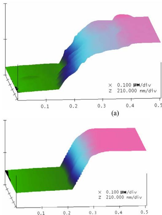
(b) Figure 3. 3D AFM images of etched mesa sidewall (a) before wet etching and (b) after wet etching. These plots were obtained with rotation angle is 85 degree and pitch angle is 10 degree.
