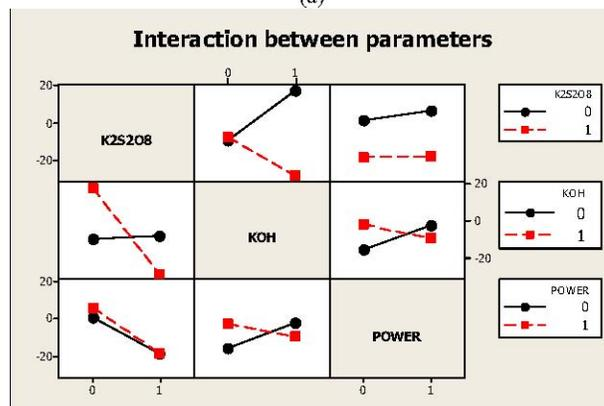
(b) Figure 1. (a) Main effects of KOH, K<sub>2</sub>S<sub>2</sub>O<sub>8</sub>, and power to surface roughness improvement (b) Interaction effects between KOH, K<sub>2</sub>S<sub>2</sub>O<sub>8</sub>, and power to surface roughness improvement.
