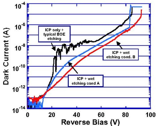
Figure 4. Reverse leakage current comparison of fabricated GaN PIN diodes grown on SiC substrate with different post-etching treatment techniques.
