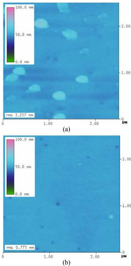
Figure 2. 2D AFM plots showing the ICP-etched n-type GaN surface (a) before the surface treatment and (b) after the surface treatment
