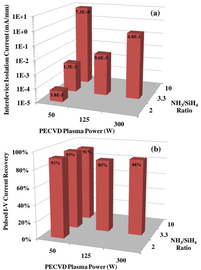
Figure 2 – (a) Interdevice isolation current density measured at  $V_{ISO} = 33V$  and (b) pulsed I-V current recovery data measured at  $V_{DG}$  QBP = 11 V for HEMTs pretreated with  $C_2F_6$  plasma and passivated with various  $SiN_x$  plasma deposition conditions.
