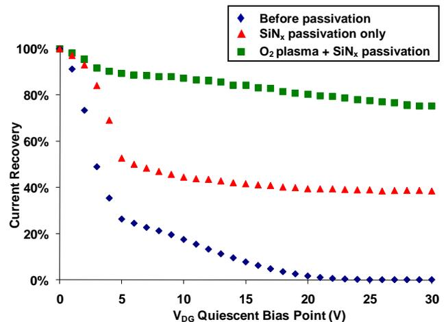
Figure 1 – Current recovery vs. V<sub>DG</sub> QBP for 1 × 100 μm<sup>2</sup> HEMTs before passivation, after SiN<sub>x</sub> passivation with no treatment, and after SiN<sub>x</sub> passivation with O<sub>2</sub> plasma treatment.
