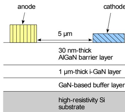
Fig. 7 Schematic cross-section drawing of the SBD.
