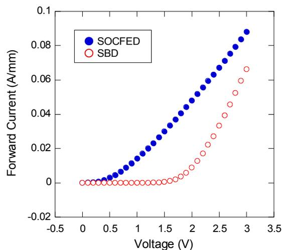
Fig. 6 Forward I-V characteristics of the SOCFED with optimized treatment condition and the SBD.
