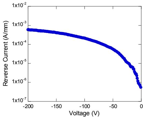
Fig. 8 Reverse I-V characteristics of the SOCFED with the optimized treatment condition.
