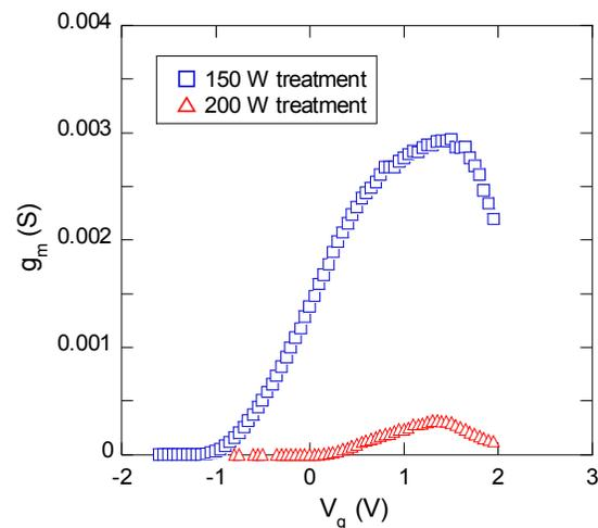
Fig. 4  $g_m$ - $V_g$  characteristics of FATFETs with the fluoride-based plasma treatment.
