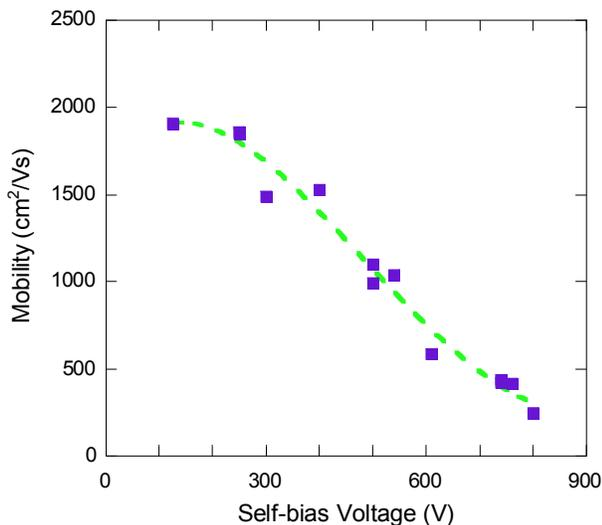
Fig. 5 Relation between the mobility of the current channel and the self-bias voltage.
