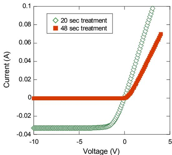
Fig. 2 Variation in the I-V characteristics of the SOCFED with fluoride-based plasma exposure time.
