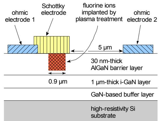
Fig. 1 Schematic cross-section drawing of the SOCFED.
