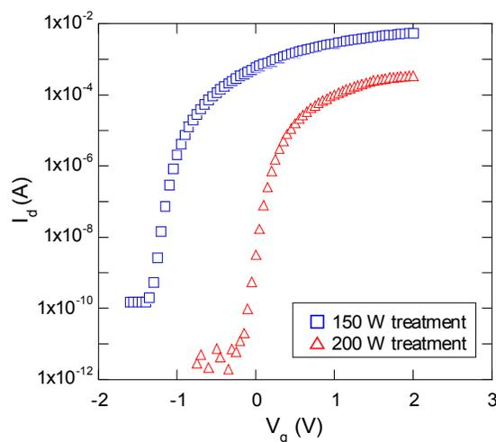
Fig. 3  $I_d$ - $V_g$  characteristics of FATFETs with the fluoride-based plasma treatment.
