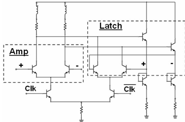
Figure 7: Circuit Implementation of Static Frequency Divider Latch, One Half of Core Circuit
