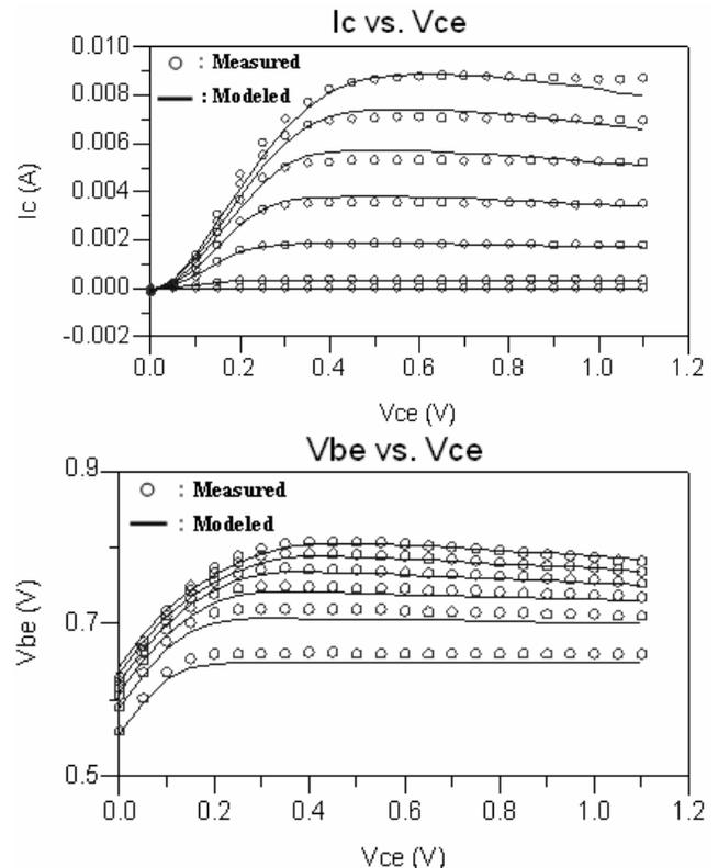
Figure 3: DC Current and Voltage Families of Device ( $I_b = 0 - 240 \mu A$ )
