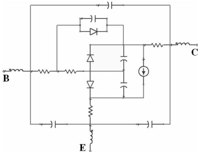
Figure 2: UIUC SDD Type-II Model Topology
