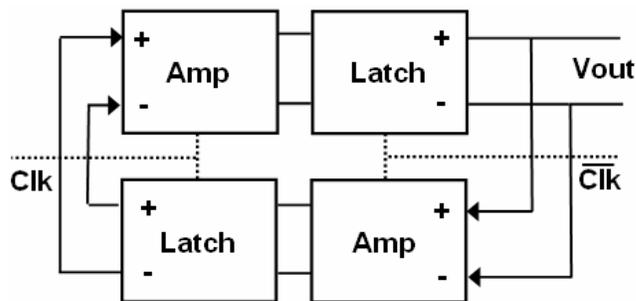
Figure 6: Block Diagram of Static Frequency Divider
