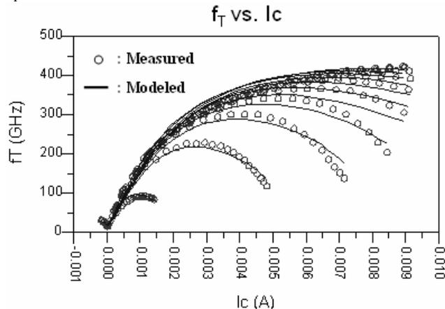
Figure 5:  $f_T$  versus Collector Current
