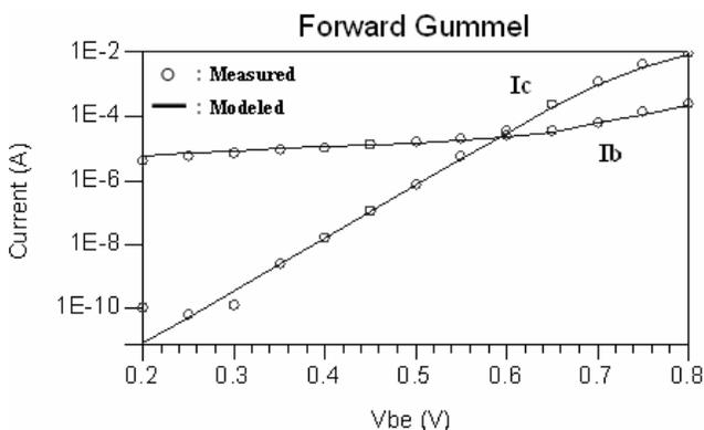
Figure 4: Forward Gummel Characteristics of Device
