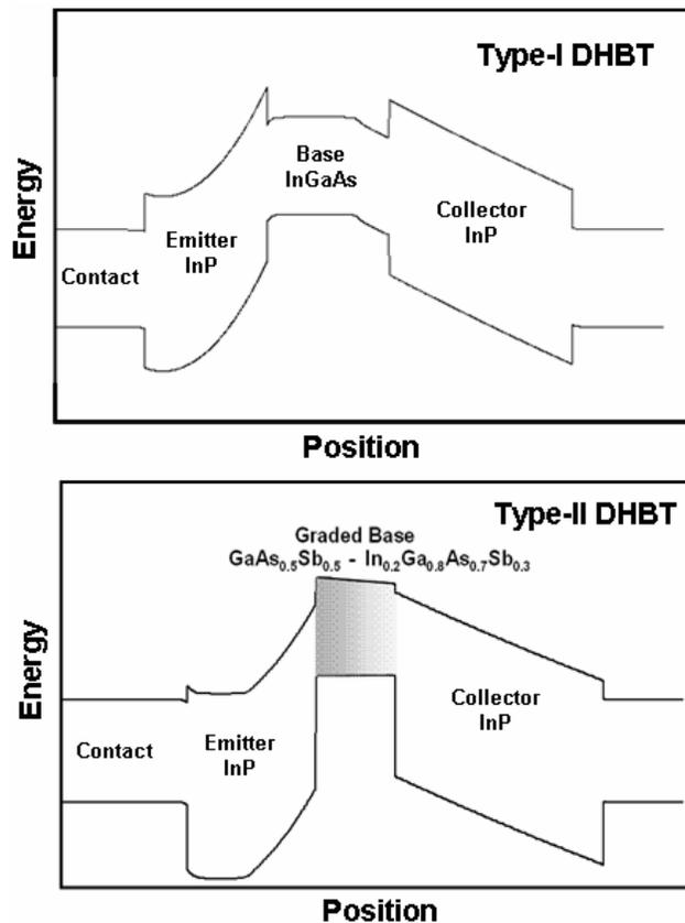
Figure 1: Type-I and Type-II DHBT Band Structures
