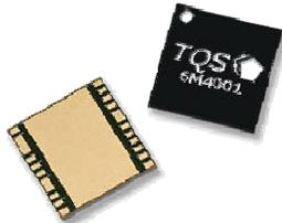
FIGURE 5. FULLY ASSEMBLED SiP MODULES
