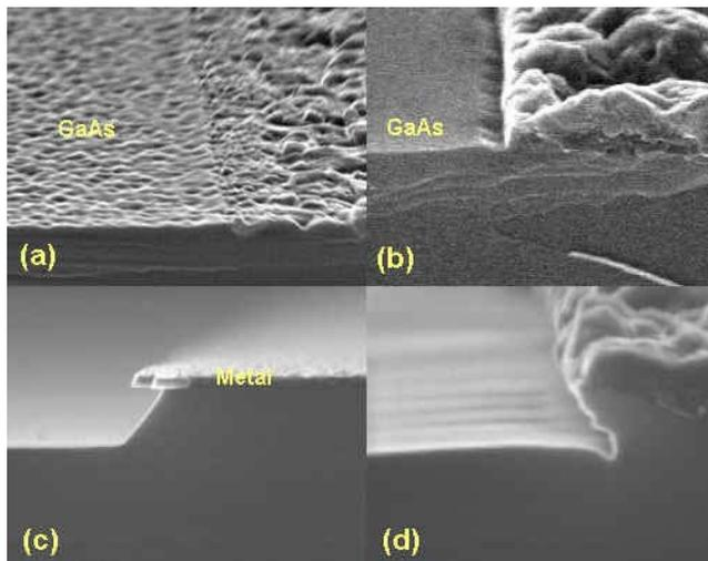
Fig 3: (a) Re-grown GaAs sample without proper cleaning. (b) Smooth re-grown GaAs surface, which is cleaned with the flow mentioned in the article. (c) Patterned GaAs with under cut (before regrowth). (d) The side profile of the re-grown sample
