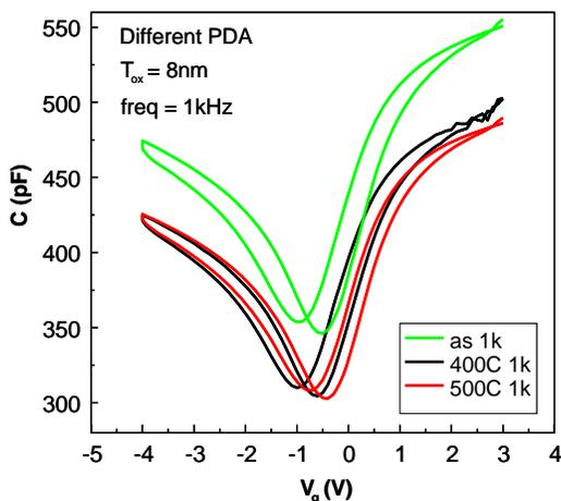
Fig 1: Quasi-static C-V curves of a 8nm  $\text{Al}_2\text{O}_3$ -ICL-InGaAs:Si-InP MOS structure measured at 1 kHz before and after annealing at 400 and  $500^\circ\text{C}$ .
