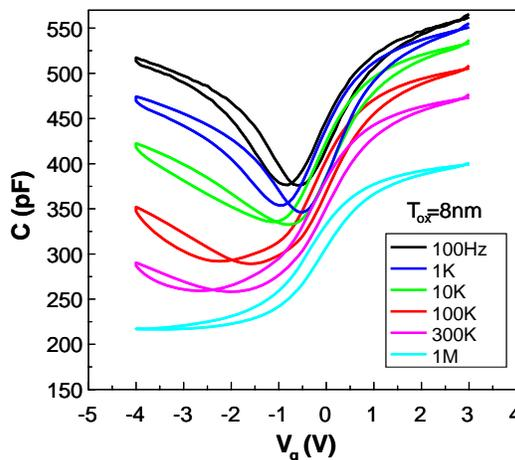
Fig 2: C-V curves of a 8nm  $\text{Al}_2\text{O}_3$ -ICL-InGaAs:Si-InP MOS structure measured 100 Hz to 1 MHz.
