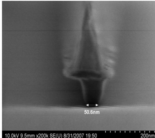
Fig 4: SEM picture of the fabricated T-gate with a 50 nm gate-length.
