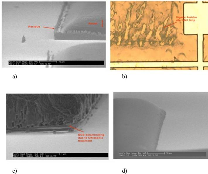
Fig.5. a) BCB Pattern after etching b) NMP – stripper could not remove cured P.R c) any stripper mix with Ultrasonic cleaning revealed BCB interface delaminating d) EKC 830 90C.
