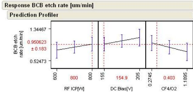
Fig.3. BCB Etch rate as function of  $CF_4 / O_2$  , ICP Power, DC Bias.
