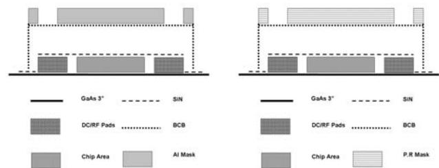
Fig.1. a) BCB etching process using Al mask (left) vs. b) Photoresist (PR) mask (right).
