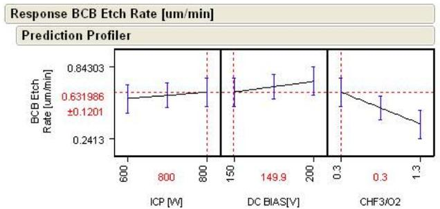
Fig.4. BCB Etch rate as function of  $CHF_3 / O_2$  ,ICP Power, DC Bias.
