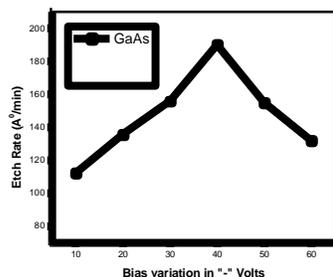
Figure 1.6 Variation of Etch rate ( $\text{\AA}/\text{min}$ ) with bias in RIE mode
