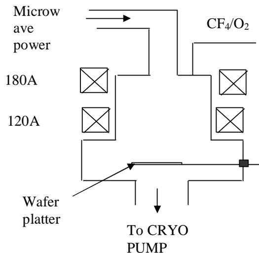
Figure 1.1 (a) Schematic of Reactive Ion Etching (RIE) mode.
