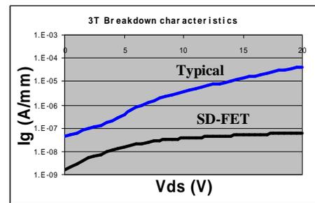
Fig. 4. Measured low gate leakage current of the SD-FET compared to that of a typical pHEMT
