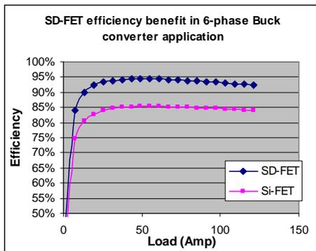
Fig. 6. Calculated SD-FET efficiency benefit in 6-phase Buck converter application
