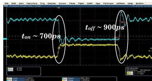
Fig. 5. Measured SD-FET turn-on and turn-off time
