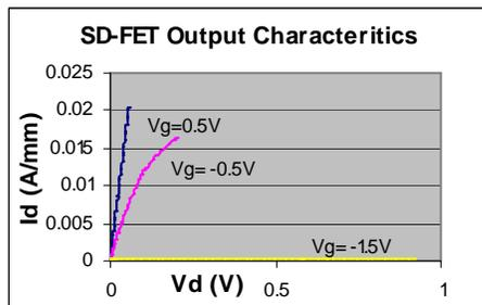
Fig. 3. Typical SD-FET output characteristics
