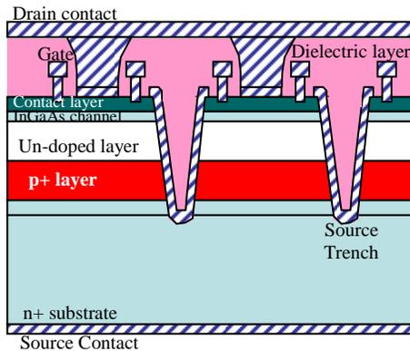
Fig. 1. Schematic of SD-FET device cross-section
