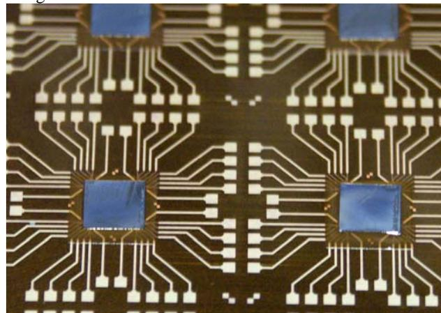
Figure 3: Example of component assembly, R2R bonded ultra-thin test chips on daisy chain test patterns on flexible PI substrates
