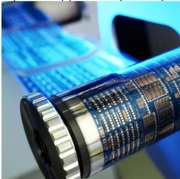
Figure 4: R2R processed flexible polymer electronic example complete roll after complete processing.
