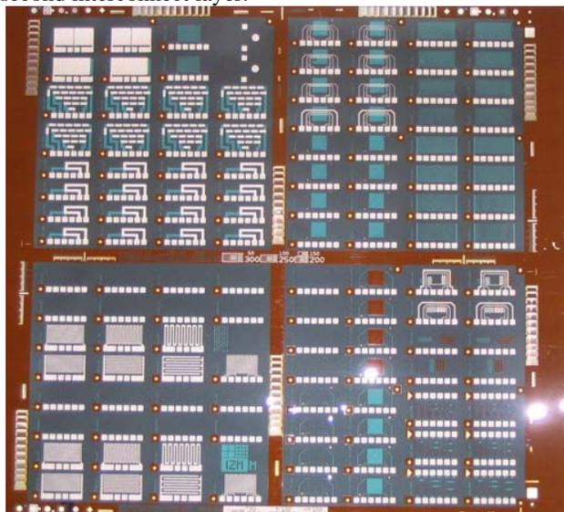
Figure 2: 2-conductor layer flex, minimal lines and spaces of lithographically structured first Cu layer:  $15\mu\text{m}$ , minimal lines and spaces of screen-printed second interconnect layer with Ag-filled-polymer:  $200\mu\text{m}$ ,  $50\mu\text{m}$  laser ablated via openings show good contact between both layers
