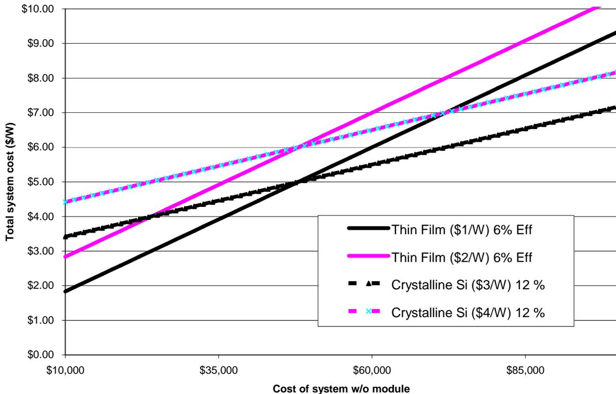
Figure 1. Calculation of system cost is presented as a function of module cost and efficiency and is plotted against the cost of the installation including all components and labor minus the PV module.
