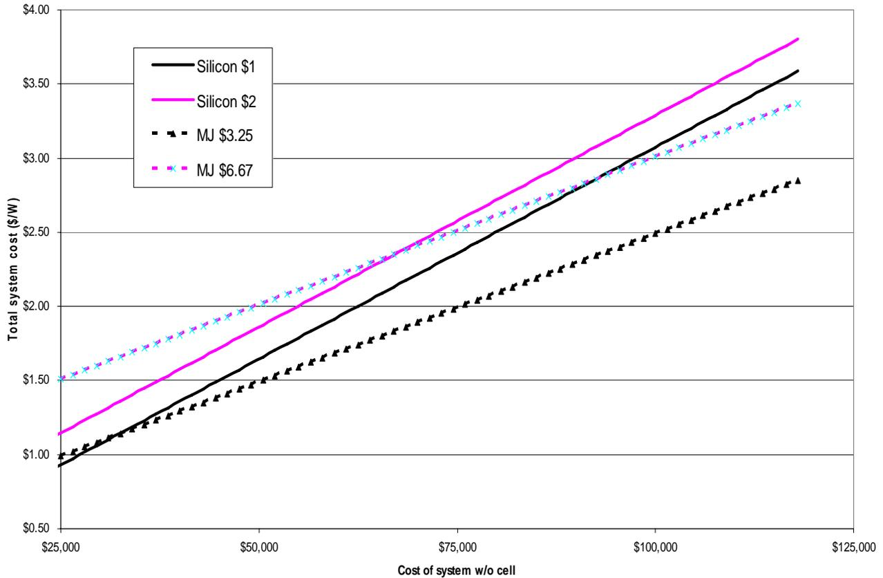
Figure 2. Calculation of system cost is presented as a function of concentrator cell cost and efficiency and is plotted against the cost of the installation including all components and labor minus the cells.
