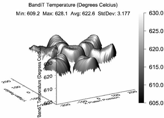
Figure 5: Surface map displaying the measured GaAs wafer temperature distribution across the seven 6" wafers in a platen. Same wafers and platen as in Fig. 4, but wider wafer backing rings cool the wafer perimeters.
