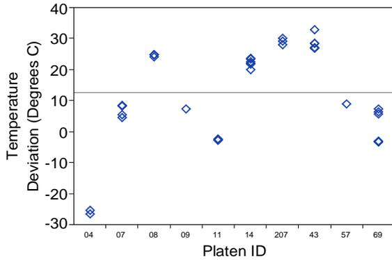
Figure 6: Oneway plot of measured temperature deviation from target. Data represents 34 MBE growth runs distributed between ten different platens of varying growth history. These temperature measurements were acquired early in each growth run prior to application of any corrective setpoint offsets.
