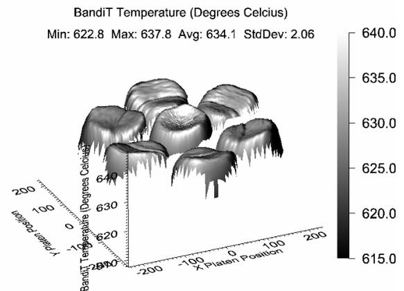
Figure 3: Surface plot displaying the measured GaAs wafer temperature distribution across the seven 6" wafers in a platen. Power supplied to the outer perimeter heat zone is 4.3% of applied manipulator heater power
