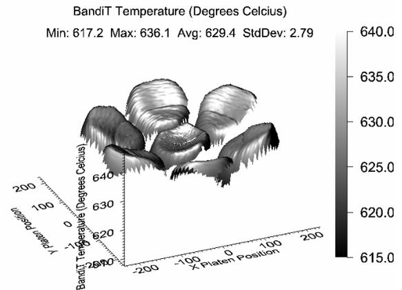
Figure 2: Surface plot displaying the measured GaAs wafer temperature distribution across the seven 6" wafers in a platen. Power supplied to the outer perimeter heat zone is 8% of applied manipulator heater power.
