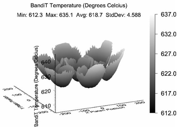
Figure 4: Surface map displaying the measured GaAs wafer temperature distribution across the seven 6" wafers in a platen. Increased contact area between wafer and platen is causing elevated temperatures at the wafer perimeters.
