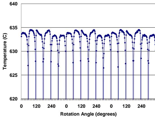
Figure 1: GaAs wafer temperature measurements during rotation of a platen of 6" GaAs wafers in 7x6" platen configuration. Data was collected from a circle ~6 inches from platen center.
