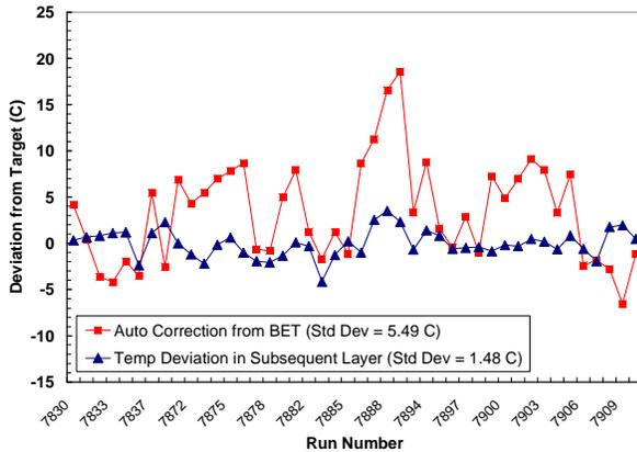
Figure 7: Trend chart showing automatic manipulator setpoint offset corrections and the resulting deviation from wafer temperature target in a subsequent layer. Data was collected from a series of 46 production epiwafer runs.
