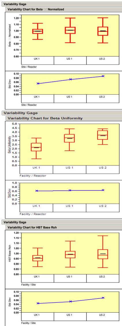
FIG 4: VARIABILITY PLOT BETWEEN REACTORS AT UK AND US FACILITIES FOR HBT DEVICE PARAMETERS. (A) CURRENT GAIN BETA, (B) BETA UNIFORMITY, (C) BASE SHEET RESISTANCE
