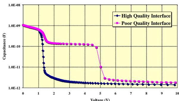
FIG 1: MESFET CV PROFILES OF ALIGNED AND UNOPTIMIZED SUBSTRATE-BUFFER INTERFACES.
