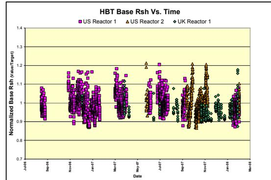
FIG 5: BASE SHEET RESISTANCE VS TIME FOR 3 REACTORS FROM TWO DIFFERENT FACILITIES.
