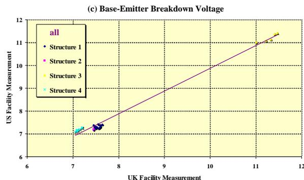
FIG 2: X-CORRELATION FOR SOME TYPICAL HBT DEVICE PARAMETERS SUCH AS (A) CURRENT GAIN BETA, (B) BASE-COLLECTOR BREAKDOWN, AND (C) BASE-EMITTER BREAKDOWN VOLTAGE.
