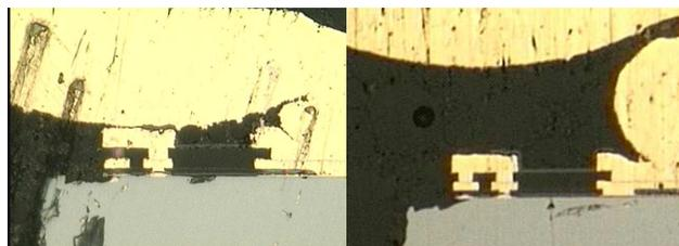
Figure 2. Cross Section of Bonded Wire Contacting Zipper (Left) and Sitting Above the Zipper (Right)
