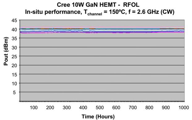
Figure 7. GaN device output power versus time showing no degradation over 1,000 hours when operated 2 dB compressed at 28 volt drain and a junction temperature of 140 °C.
