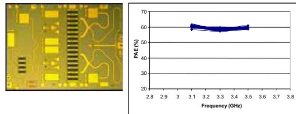
Figure 10. 40-watt 2-stage S-band GaN MMIC with 25 dB of associated gain with 60% PAE from 3.1 GHz to 3.5 GHz
