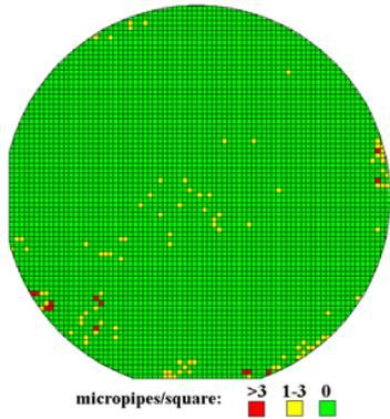
Figure 2. Micropipe map made by optical transmission microscopy showing an average micropipe density of 2.5 cm<sup>-2</sup>.
