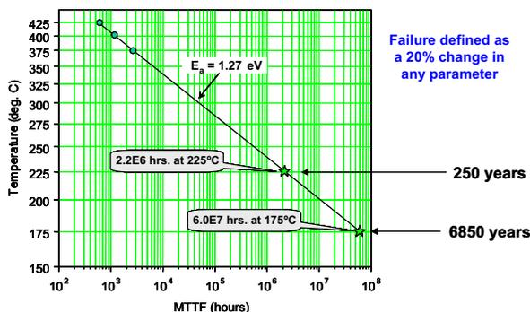
Figure 6. SiC MESFET reliability showing 2.2E6 MTTF at 225 °C junction temperature
