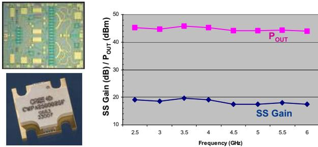
Figure 8. 2-stage GaN HEMT MMIC provides 25 watts of RF output power from 2.5-6GHz with 18 dB of small signal gain at 28 volts.
