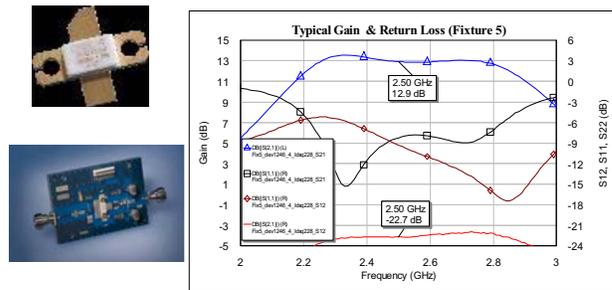
Figure 4. Cree GH27060F in a broadband application circuit designed for BWA applications
