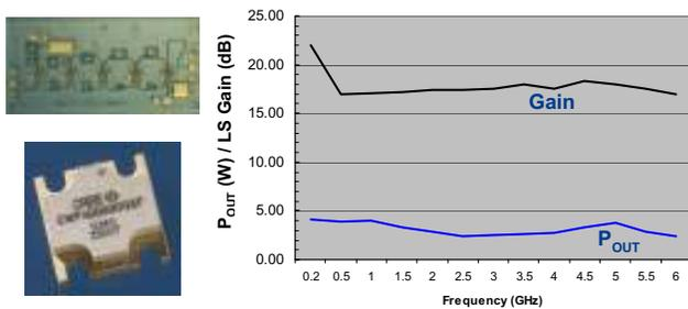
Figure 9. 3-watt packaged GaN HEMT MMIC amplifier with >17 dB of gain from 20 MHz to 6.0 GHz
