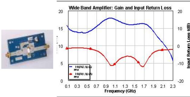
Figure 5. Cree CGH40045FF in a wideband application circuit designed for general purpose applications
