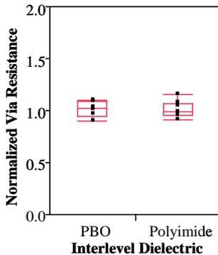
Fig. 8. Comparison of 3.0µm via resistance with PBO and polyimide as interlevel dielectric.
