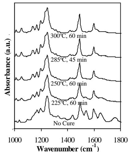
Fig. 1. FTIR spectra of PBO before and after cured at various conditions.
