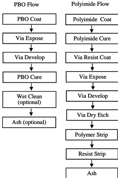
Fig. 2. Comparison between PBO and polyimide interlevel dielectric process flows.
