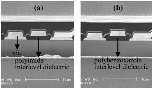
Fig. 7. FIB/SEM images of the vias on top of metal lines with (a) polyimide and (b) PBO, as interlevel dielectric.
