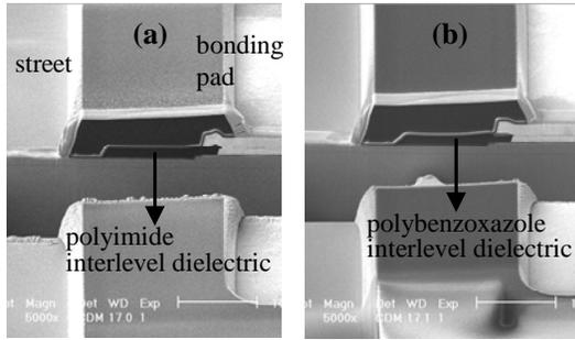
Fig. 6. FIB/SEM images of the bonding pad and street area with (a) polyimide and (b) PBO, as interlevel dielectric.
