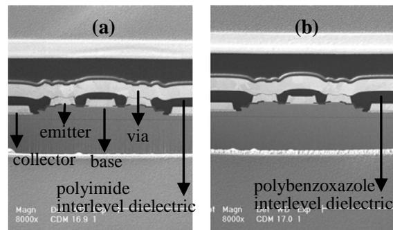
Fig. 5. FIB/SEM images of the HBT area with (a) polyimide and (b) PBO, as interlevel dielectric with the vias on top of the emitter.
