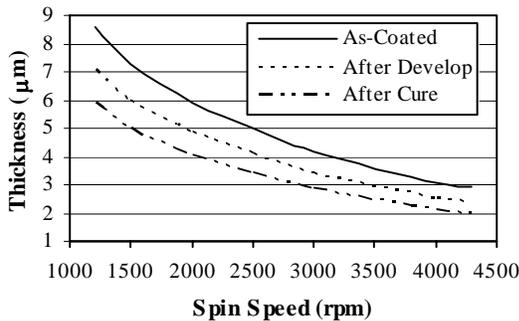
Fig. 3. Spin-speed curve of PBO as-coated, after develop, and after cure.
