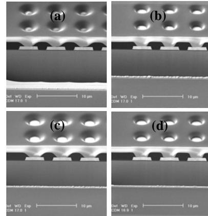
Fig. 4. FIB/SEM images of 3.0 $\mu$ m vias with exposure energy/focus conditions of (a) 500mJ/-3.0 $\mu$ m, (b) 500mJ/+1.0 $\mu$ m, (c) 800mJ/-3.0 $\mu$ m, and (d) 800mJ/+1.0 $\mu$ m.
