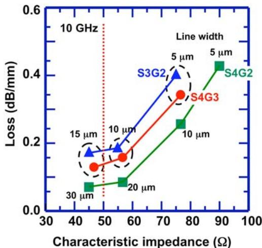
Fig. 8. Dependence of loss on the characteristic impedance for the three TFMS line structures.
