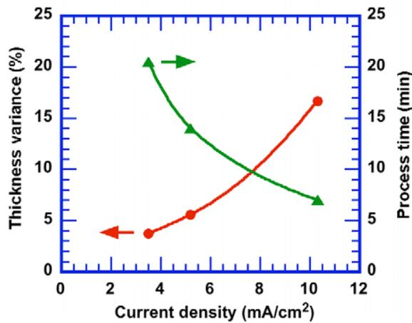
Fig. 5. Dependence of thickness variance and process time on current density for plated Au with 5- $\mu\text{m}$  thickness.
