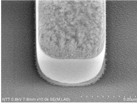
Fig. 4. SEM image of the 4th Au metal layer with 5- $\mu\text{m}$  thickness and 6- $\mu\text{m}$  width, formed by electroplating.
