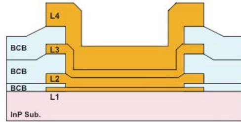
Fig. 6(a). Cross-sectional view of the pad stack structure without BCB films between two metal layers.
