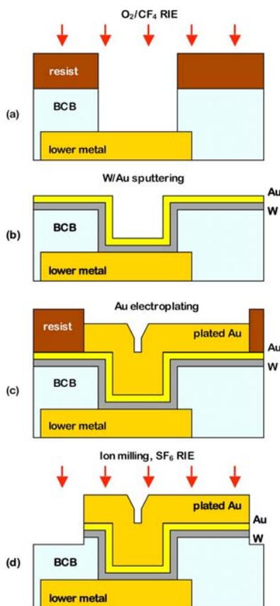
Fig. 2. Main steps of the fabrication process.
