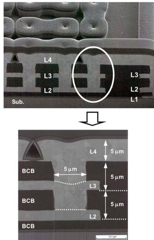
Fig. 1. Cross-sectional microphotograph of the four-level interconnect structure.
