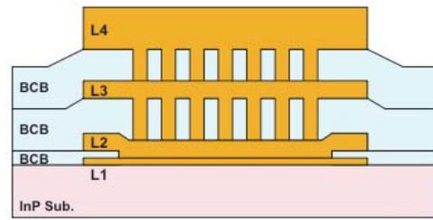
Fig. 6(b). Cross-sectional view of the pad stack structure with via-contact array.
