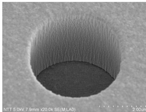
Fig. 3. SEM image of a via-hole with a diameter of 4  $\mu\text{m}$ , which is coated with a thin metal layer.
