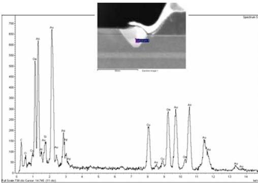
Figure 4: EDS at the diffused metal showing dominant Au peak
