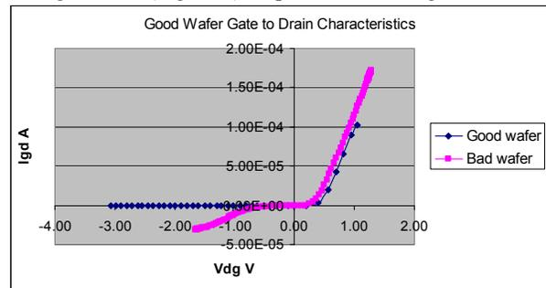
Figure 1: Bad wafer showing higher leakage than good wafer
