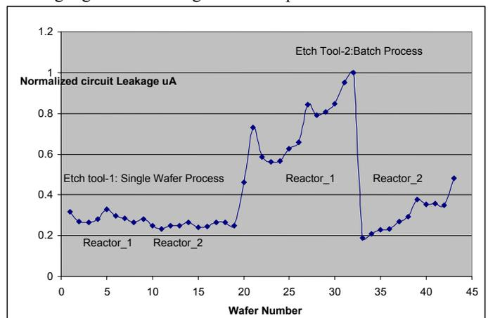
Figure 16: Circuit leakage affected by MBE reactors and etch tools.
