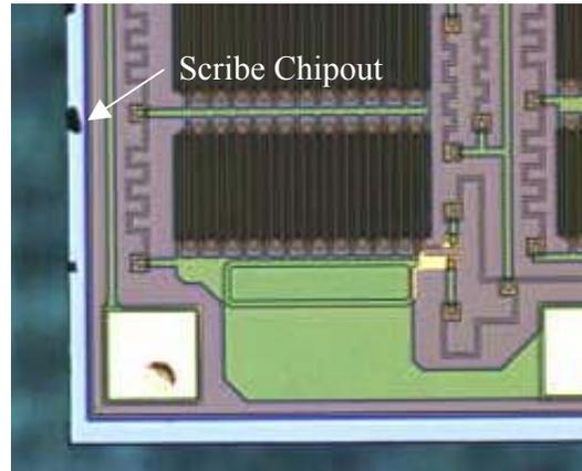
Figure 5 Picture showing scribe chip out
