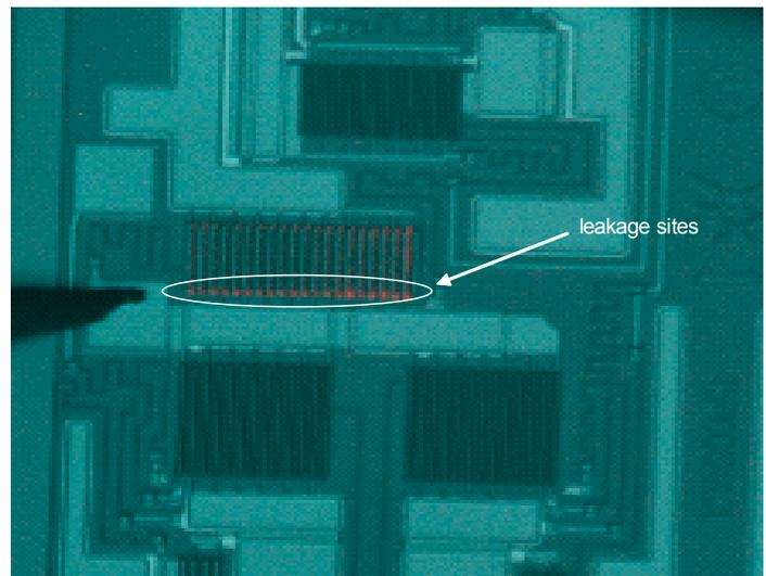
Figure 2 Photoemission imaging showed hot spots of leakage current
