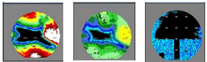
Figure 17: Examples of invalid Insertion Loss, Isolation, & 3<sup>rd</sup> harmonic tests. Failing sites are black
