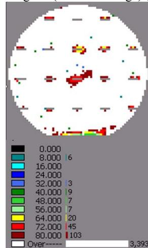
Figure 6 Parameter Viewer map of leakage current
