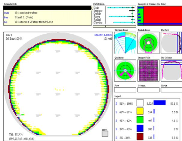
Figure 11 *dataPOWER®* stacked wafer yield map showing yield loss due to probe card
