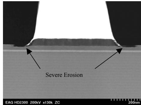
Fig. 13 FIB-TEM illustrating erosion around gate
