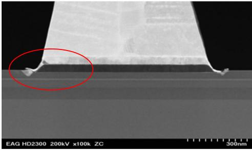
Figure 3: FIB-TEM on leaky device
