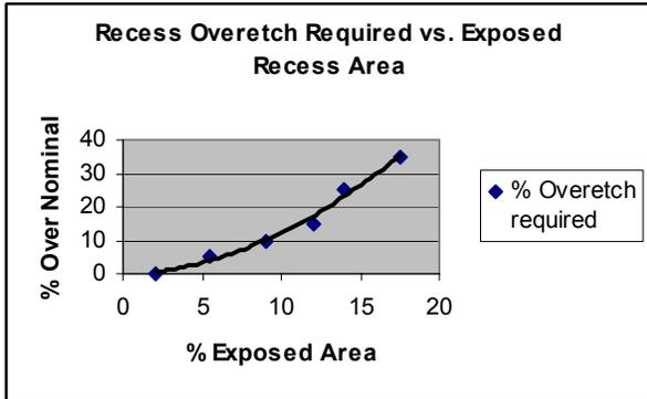
Figure 7 Required over-etch vs. exposed area.
