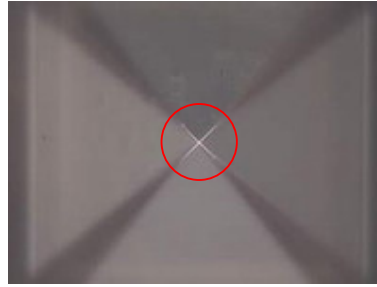
Fig.4. The tip profile of a 4-point tool.
