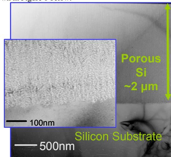
Figure 1. TEM showing formation of porous silicon layer. The dendritic nature of the porous layer is shown in the inset.
