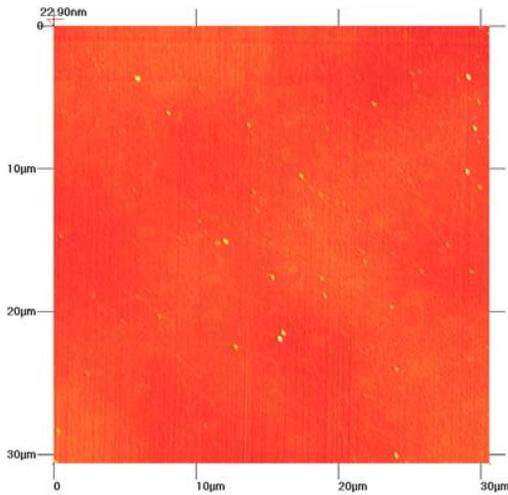
**Figure 2(b).** Surface of SiN-coated porous Si.  $\sim 0.5$  nm r.m.s. roughness. The particulates on the surface were introduced during the AFM measurement and are easily removed during subsequent processing.
