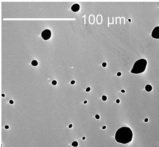
**Figure 5.** Cleaved surface of annealed porous silicon showing large pores that controllably weaken the material to produce a facile fracture interface.
