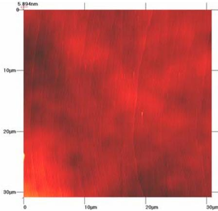
**Figure 2(a).** Surface of porous silicon. The r.m.s. roughness is  $\sim 0.5$  nm.
