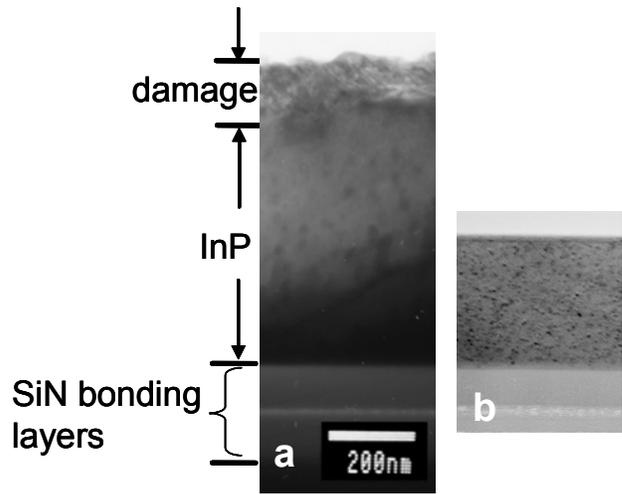
**Figure 3.** CMP of InP transferred layers. (a) prior to polishing, there is residual damage from the implant process. (b) after CMP, the damaged material is removed and the surface roughness is  $0.5$  nm r.m.s. The speckle observed in the InP layers is related to TEM sample preparation damage.
