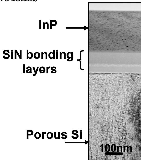
**Figure 4.** TEM of CELT substrate with InP template layer, silicon nitride bonding layers, and a porous silicon substrate.
