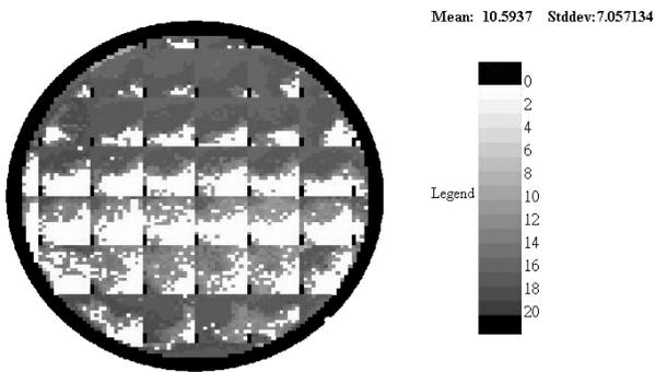
Figure 5 shows the reticle-dependent wafer map of the measured breakdown voltage distribution across a six-inch wafer.
