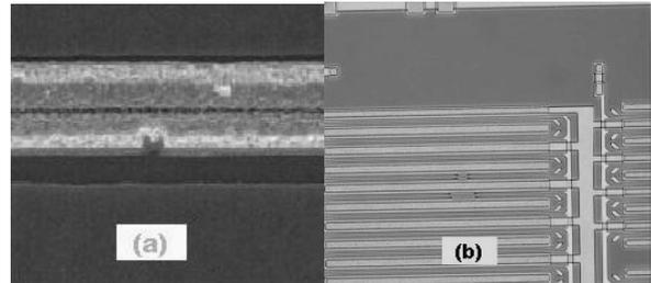
Figure 1 (a) defective gate and 1 (b) broken gate fingers.
