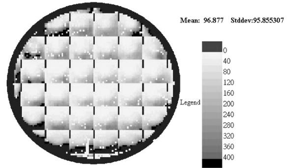
Figure 6 shows the reticle-dependent wafer map of the measured drain transient time distribution across a six-inch wafer.
