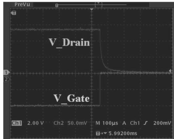
Figure 7 shows the drain transient time test result from the oscilloscope.
