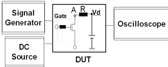
Figure 2: Test system setup.
