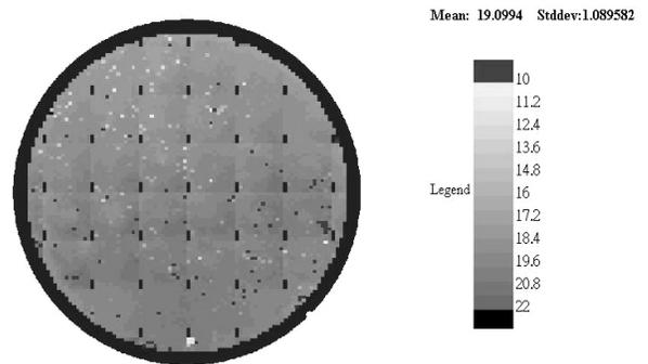
Figure 8 shows the wafer map for breakdown voltage after the gate process parameters were re-optimized.
