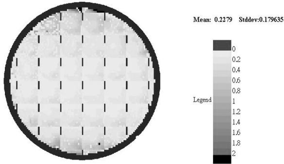
Figure 9 shows the wafer map for drain transient time after the gate process parameters were re-optimized.
