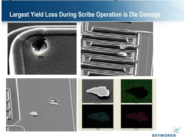
**Figure 7: Damage Caused by Undocumented "Improvement"**
