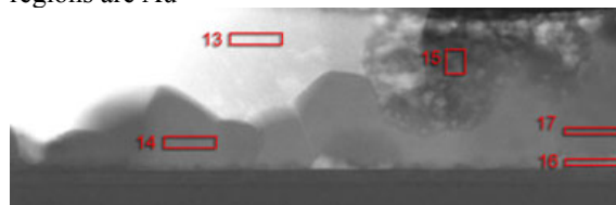
Figure 6 Group A. New ohmic. 380C, 10sec
