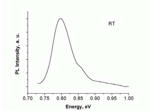
Fig. 1: PL spectrum taken at RT of 5-stack QDH structure.
