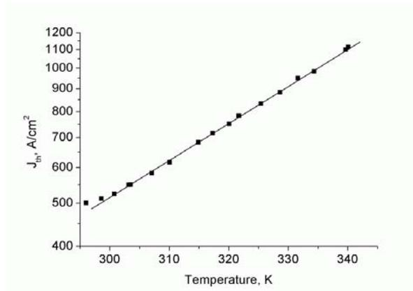
Fig. 4:  $J_{th}$  as a function of temperature for 5-stack QDH laser.
