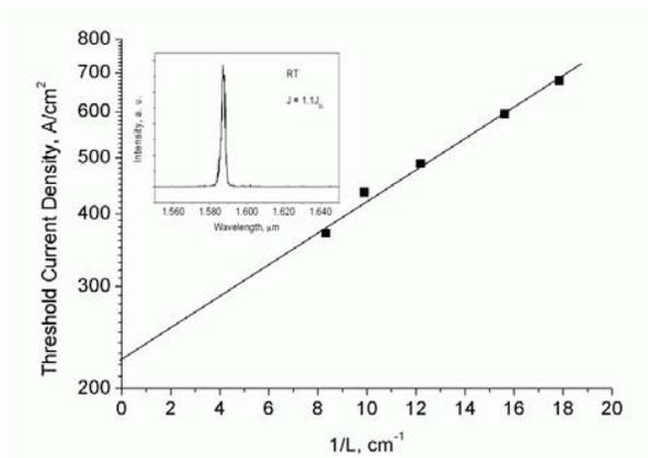
Fig. 2:  $J_{th}$  vs the reciprocal length taken at RT for 5-layer stacked QDH lasers. The inset shows a lasing spectrum at  $1.1 \times J_{th}$  for a cavity length of 1.2 mm.
