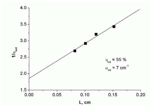
Fig. 3: Inverse external quantum efficiency vs cavity length taken at RT.
