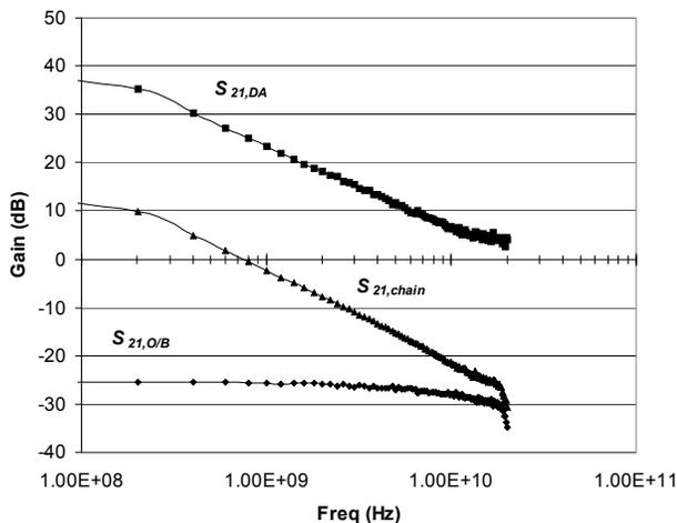
Fig. 6 Measured  $S_{21}$  of amplifier chain and output buffer test circuits at high frequencies. Scalar determination of diff amp gain is determined as  $S_{21,DA} = S_{21,chain} - S_{21,O/B}$ . Core diff amp utilized  $3-2 \times 5 \mu m^2$  HBT in each diff amp branch with 6-finger  $2 \mu m$  PMOS devices.  $I_{SS} = 10mA$ ,  $V_{SS} = -6V$ .
