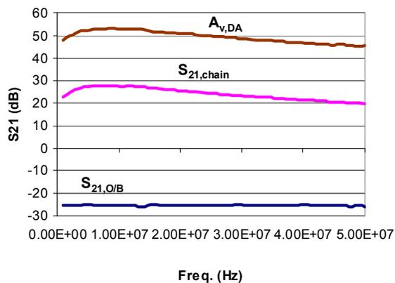
Fig. 7 Measured  $S_{21}$  of amplifier chain and output buffer test circuits at low frequencies. Low frequency gain  $A_{V,DA}$  is given by  $A_{V,DA} = S_{21,chain} - S_{21,O/B}$ . Core diff amp utilized  $3-2 \times 5 \mu m^2$  HBT in each diff amp branch with 6-finger  $2 \mu m$  PMOS devices.  $I_{SS} = 10mA$ ,  $V_{SS} = -6V$ .
