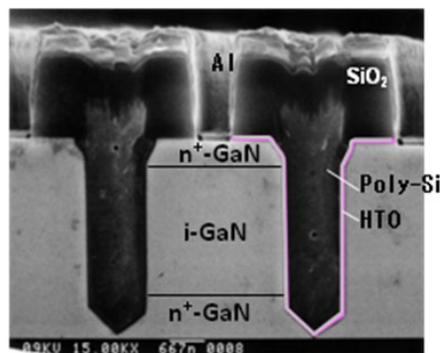
Fig.5. The cross-sectional photograph of the UMOSFET
