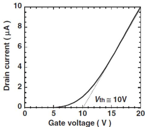
Fig.8 Typical I<sub>D</sub>-V<sub>G</sub> characteristics under drain voltage of 0.1V.
