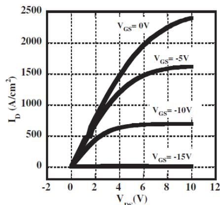
Fig.3 I<sub>D</sub>-V<sub>DS</sub> characteristics of the vertical insulated gate AlGaN/GaN HFET
