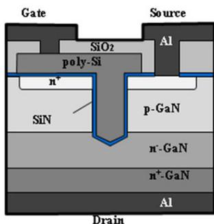
Fig.7 The schematic cross-sectional view of the UMISFET.
