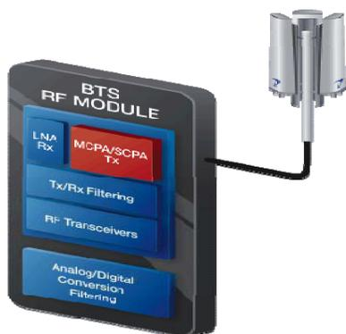
Figure 1. Typical BTS Block Diagram
