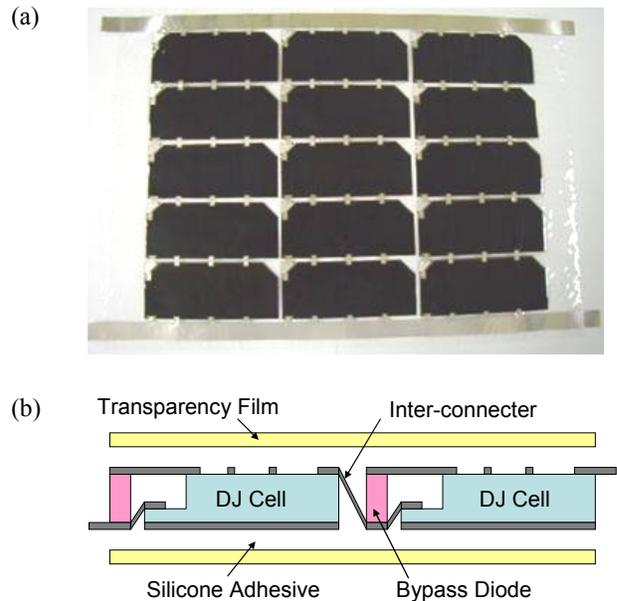
Figure 5: (a) Photograph of space solar sheet and (b) schematic cross section view.
