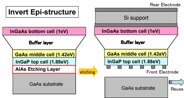
Figure 9: Cell fabrication process to realize high efficiency InGaP/GaAs/InGaAs(1eV) triple-junction cell.
