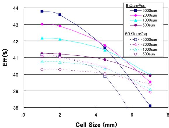
Figure 6: Increase in efficiency by reducing cell size, as a dependence of sheet resistance. (Calculation)
