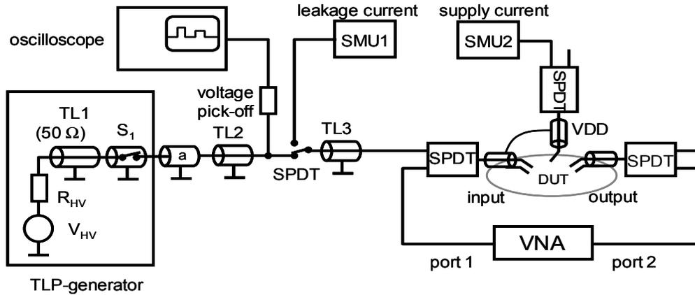
Figure 1: Measurement set-up of the RF-TLP system
