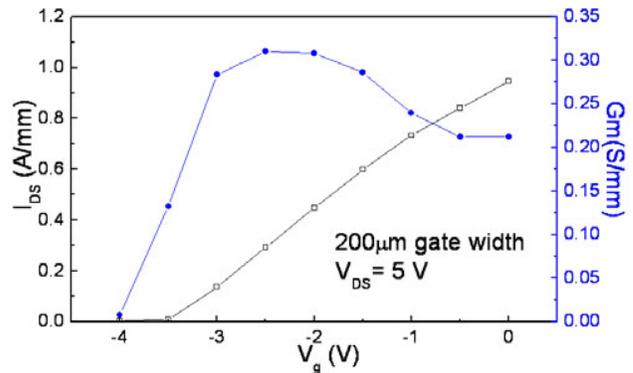
Figure 7.  $I_{DS}$  and extrinsic transconductance of an AlN/GaN HEMT with a gate dimension of  $0.38 \times 200 \mu\text{m}^2$ .
