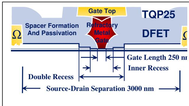
Figure 1: Schematic Cross-Section of a TQP25 DFET.
