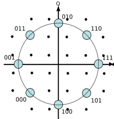
**Figure 1. A 32-QAM Constellation for Evolved LTE EDGE with overlay of 8-PSK showing the increased linearity requirement.**
