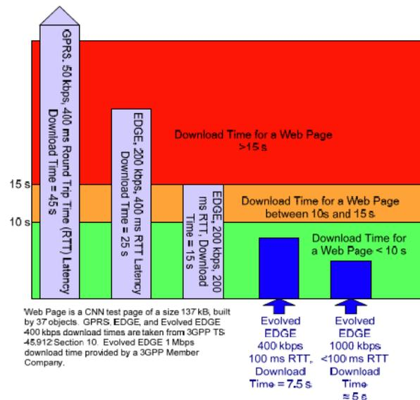
Figure 4. Web page download times as a function of technology. Source: Global Mobile Suppliers Association[2].
