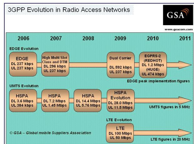
**Figure 2. Time line and network speeds for evolving cellular technologies[2].**
