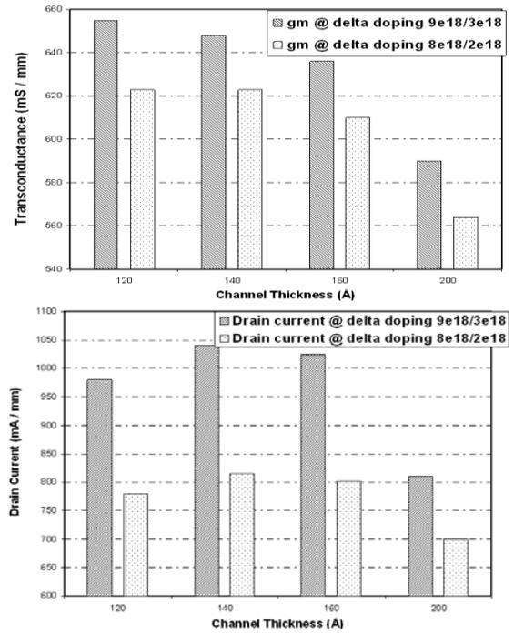
Fig 4:  $I_D$  and  $g_m$  vs. channel thickness of penta-composite MHEMT with two different  $\delta$ -doping
