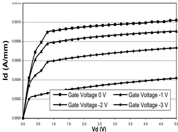
Fig 3:  $I_D$  vs  $V_D$  curve of 140Å InAlAs/InGaAs MHEMT
