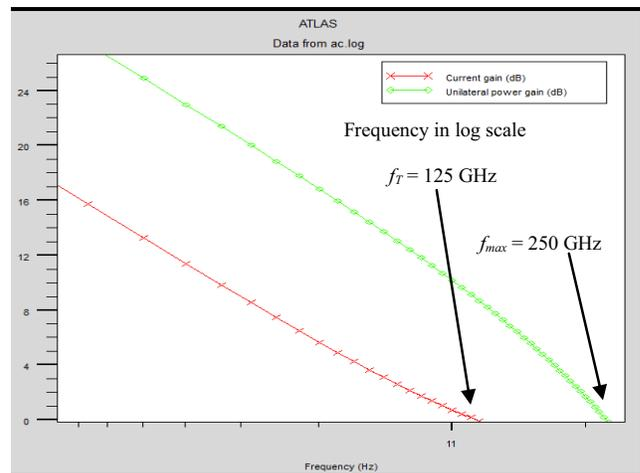
Fig 5: Frequency response of 140 Å InAlAs/InGaAs penta-channel HEMT
