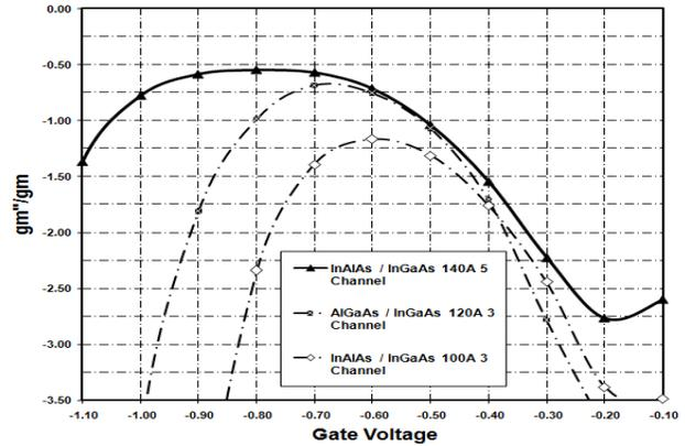
Fig 7: Comparative study of IP3 of MHEMT and PHEMT
