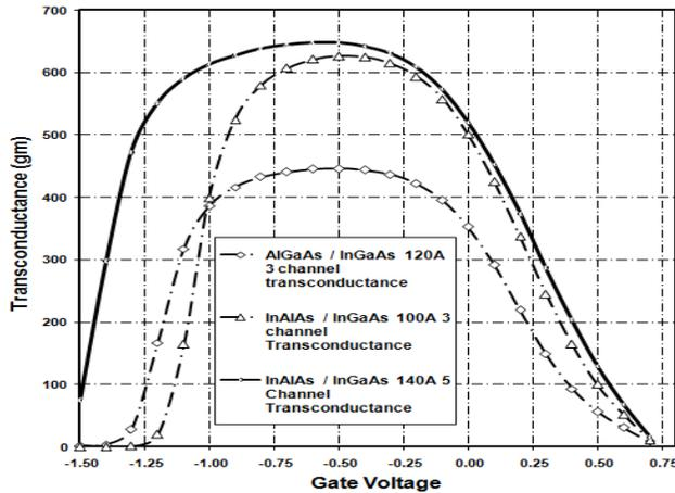
Fig 6: Comparative study of  $g_m$  curve of penta and tri-composite channel InAlAs/InGaAs MHEMT and AlGaAs/InGaAs PHEMT
