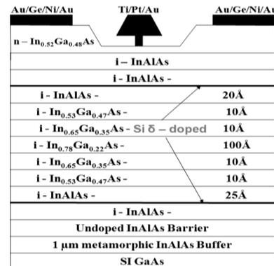
Fig 1:  $\text{In}_{0.78}\text{Ga}_{0.22}\text{As}$  penta-composite channel structure MHEMT
