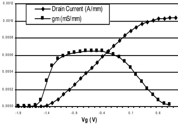
Fig 2:  $I_D$  &  $g_m$  vs  $V_D$  curve of 140Å InAlAs/InGaAs MHEMT
