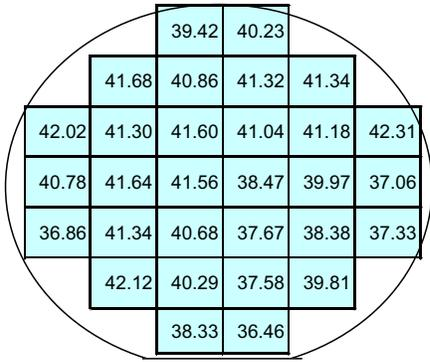
Figure 3. Typical current gain wafer map of a  $0.8 \times 3 \mu\text{m}^2$  DHBT3 at  $J_c = 100 \text{ kA/cm}^2$ .
