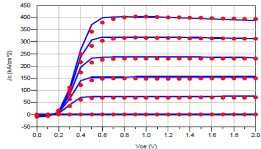
Figure 2. Typical IV curves of a 0.8x5 μm<sup>2</sup> InP DHBT3 device. Solid lines are measured data and dots are modeled data.
