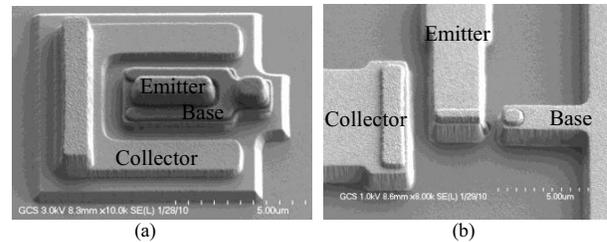
Figure 1. SEM pictures of a 0.8x3μm<sup>2</sup> DHBT, (a) prior to BCB passivation, (b) posts and first level interconnect metal.
