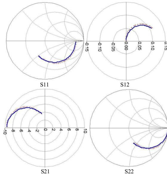
Figure 7. Measured (solid line) and modeled (dots) s-parameters for a 0.8x5  $\mu\text{m}^2$  DHBT3 device at  $J_c=200\text{kA/cm}^2$  and  $V_{ce}=1.5\text{V}$  in frequency range from 0.5 to 40GHz.
