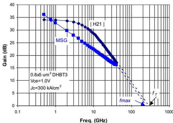
Figure 4.  $|H_{21}|$  and MSG/Gmax vs frequency for a  $0.8 \times 5 \mu\text{m}^2$  InP DHBT3 device at  $V_{ce} = 1.0 \text{ V}$  and  $J_c = 300 \text{ kA/cm}^2$ .
