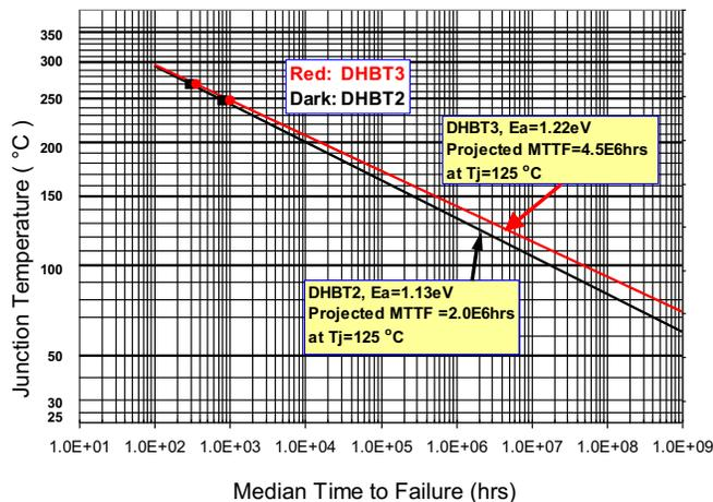
Figure 10. Arrhenius plots for both DHBT2 and DHBT3 at two temperatures. Extrapolated MTTF  $> 2 \times 10^6$  hours at  $T_j = 125^\circ C$  and  $E_a > 1.1eV$ .
