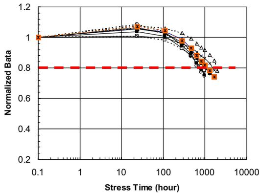
Figure 8. Normalized beta vs high temperature stress time of 10 DHBT3 devices at  $V_{ce}=1.25V$ ,  $J_c=300kA/cm^2$  and  $T_j=248^\circ C$ .
