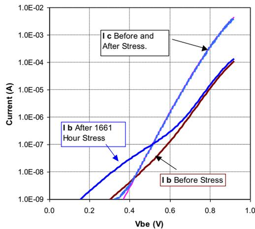
Figure 9. Gummel plots of a  $0.8 \times 5 \mu m^2$  DHBT device before and after 1661 hour stress.
