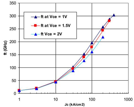
Figure 5.  $f_T$  vs  $J_c$  for a  $0.8 \times 5 \mu\text{m}^2$  InP DHBT3 device at  $V_{ce} = 1.0, 1.5,$  and  $2.0 \text{ V}$  at room temperature.
