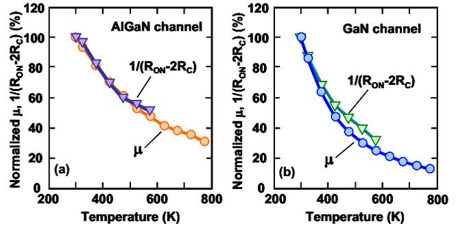
Fig.6 Normalized Hall mobility and the inverse of ( $R_{ON} - 2R_C$ ) as a function of temperature for AlGaIn-channel HEMT (a) and for GaN-channel HEMT (b).
