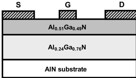
Fig.1 Schematic cross-sectional structure of Al<sub>0.51</sub>Ga<sub>0.49</sub>N/Al<sub>0.24</sub>Ga<sub>0.76</sub>N HEMT on AlN substrate.
