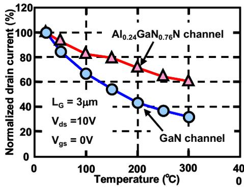
Fig.4 Normalized drain current as a function of temperature for AlGaIn-channel HEMT and for GaN-channel HEMT.
