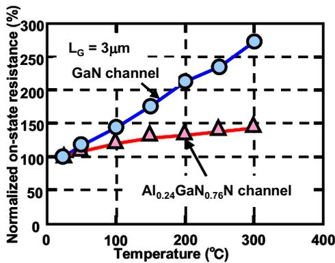
Fig.5 Normalized on-state resistance as a function of temperature for AlGaIn-channel HEMT and for GaN-channel HEMT.
