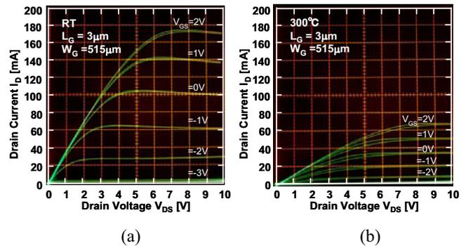
Fig.3 Drain I-V characteristics for Ga<sub>N</sub>-channel HEMT measured at RT (a) and at 300°C (b).
