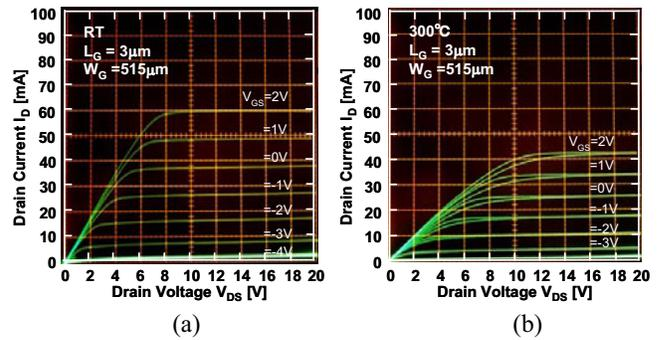
Fig.2 Drain I-V characteristics for AlGa<sub>N</sub>-channel HEMT with Al composition of 0.24 measured at RT (a) and at 300°C (b).
