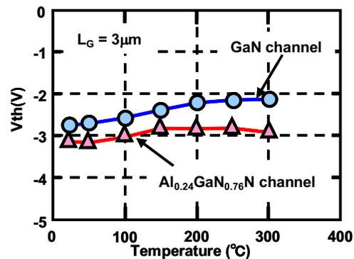
Fig.7 Threshold voltage as a function of temperature for AlGaIn-channel HEMT and for GaN-channel HEMT.
