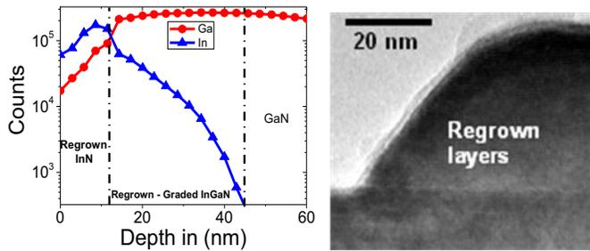
Fig.4(a) SIMS measurements showing graded InGaN and InN cap
