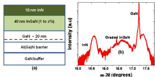
**Fig. 3** (Color online) (a) Epitaxial structure of the samples with 40 nm InGaN graded from 1% to A (30%), B (54%) and C (63%) and 10 nm InN cap (b) HRXRD ( $\omega$ -2 $\theta$ ) for sample C with peaks corresponding to regrown InN and graded InGaN indicated.
