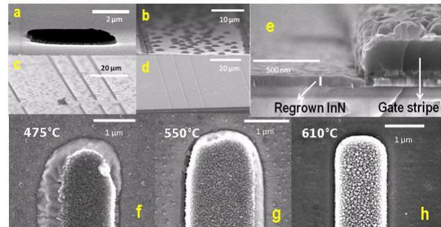
**Fig. 2(a-e)** Top view scanning electron micrographs of InN source-drain regions regrown at growth temperatures of (a) 575°C, (b) 525°C, (c) 500°C and (d) 475°C. (e) Cross-section SEM image of regrown InN source-drain region next to the gate stripe (**f-h**) Top view scanning electron micrographs of regrown graded InGaN layers grown at (f) 475°C (g) 550°C (h) 610°C
