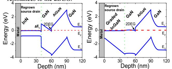
**Fig. 1** (a) Simulated band diagram of InN regrown source drain to a N-polar GaN HEMT. The high  $\Delta E_c$  at the InN and GaN interface is a barrier to the flow of electrons from the metal to the 2DEG. (b) Simulated band diagram of InGaIn graded from GaN  $\rightarrow$  InN for source drain regions of a N-polar GaN HEMT.
