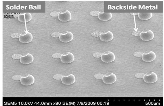
Figure 3 Solder Ball Array On Top Of GaAs Wafer Backside Metallization. Final ball height is about 90um
