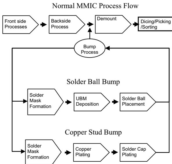
Figure 1 Wafer Level Bump Integration Process Flow
