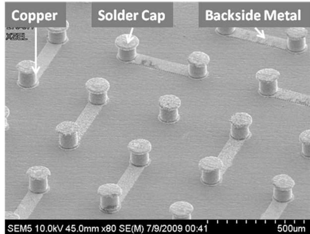
Figure 2 Electroplated Copper Studs Covered With Thin Solder Cap On Top of GaAs Wafer Backside Metallization. Total bump height 100um
