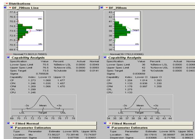
Figure 8: Process capability of AZ5510 printing features of 700nm and 350nm
