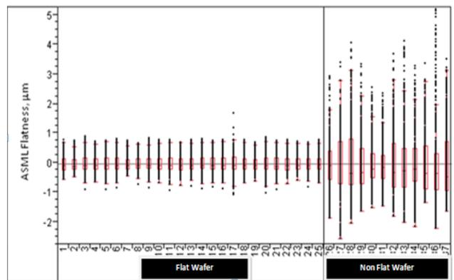
Figure 4: Mapping of wafer flatness for the incoming wafer
