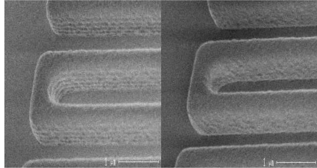
Figure 3: Standing waves which can be suppressed with a bottom anti reflective coating
