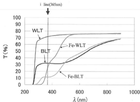
Figure 2: Transmittance varies significantly at 365nm for differing substrates used in the manufacture of SAW filters
