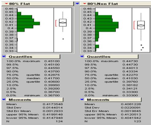
Figure 5: Comparison of line size across wafer for a flat and non flat wafer
