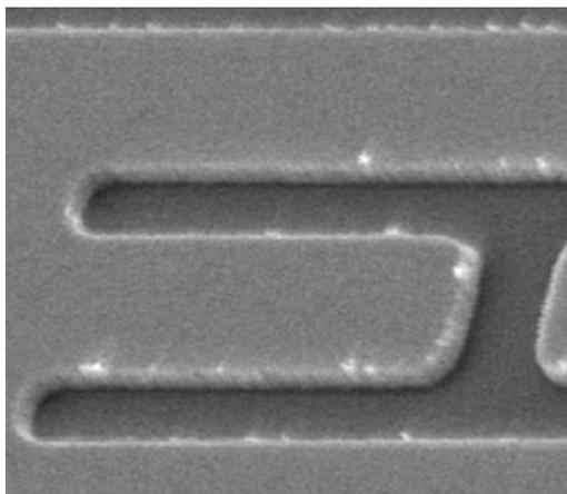
Figure 6: Metal 'wings' which are detrimental to device performance
